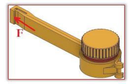
Figure 6. The acting force of the finger
