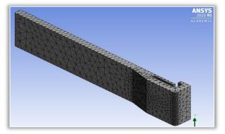
Figure 8. Tetrahedron mesh (fine and coarse)
