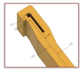
Figure 4. Wall thickness
