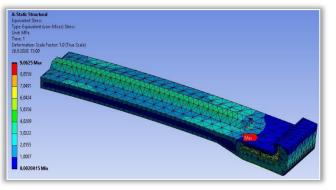
Figure 9. The Von-Mises Stress distribution
