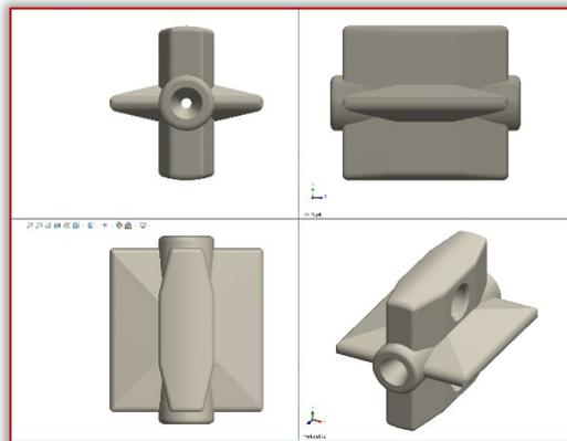
Figure 5. 3D model of the piece, from different angles, in the SolidWorks software. In Figure 6 one can see how the STL model fully reproduces the geometry of the part, made in the SolidWorks software.
