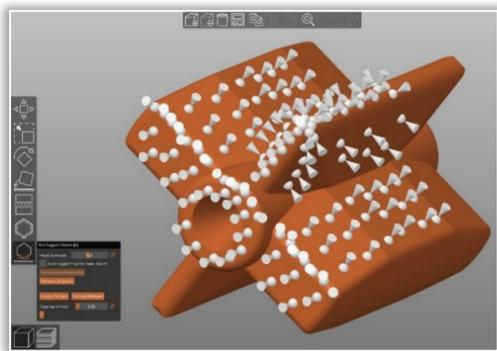
Figure 7. Manual application of the support layers
