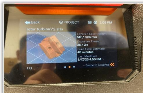
Figure 10. 3D printing parameters of the part
