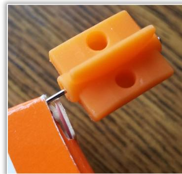
Figure 14. The final result of the entire process – the fully functional flowmeter rotor
