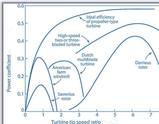
Figure 1. Power coefficient for different types of turbines [10]
