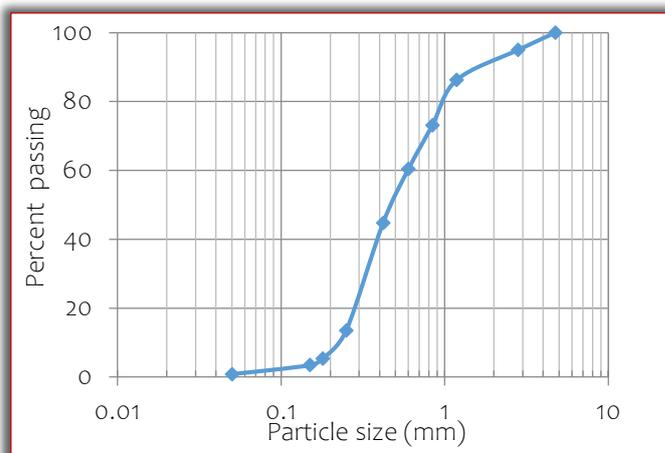
Figure 1. Particle size distribution of river sand
