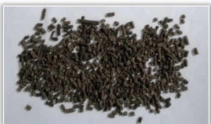
Figure 1 – Granular fertilizer material based on biosolids a) –variant V1, b)–variant V2
