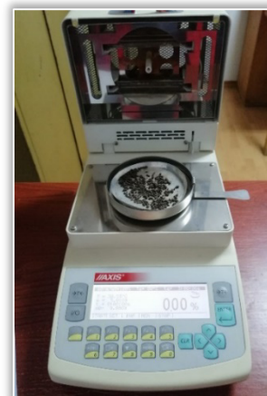
Figure 2 – Determination of moisture content with thermobalance AXIS –100
