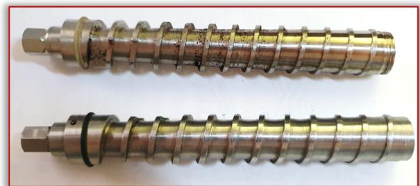
Figure 4 – Two screws with different pitches
