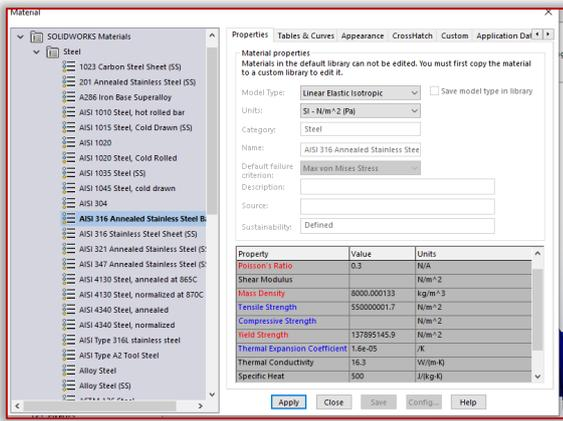
Figure 5b – Material properties AISI 316 – Stainless Steel
