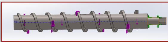
Figure 6 – 3D model of screw
