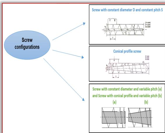
Figure 2 – Multiple models of the screw (V.V. Jinescu, 2007, P. Sari, 2006)
