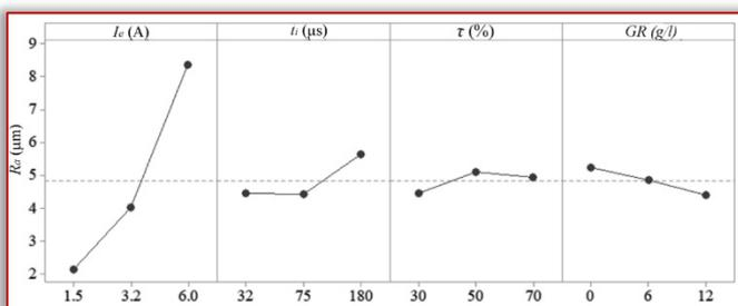
Figure 3. Response ANOVA graph for the Ra
