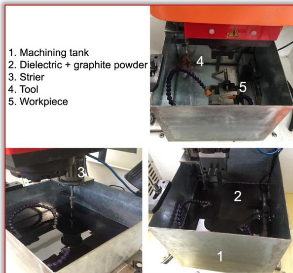
Figure 1. Setup of PMEDM.
