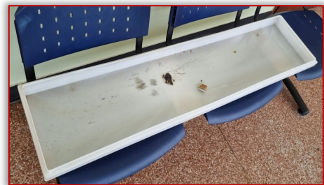
Figure 6. The diffuser of the lighting fixture and pieces of the plastic housing of the ballast previously observed by thermographic inspection
