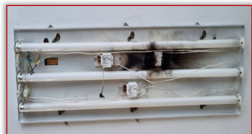
Figure 6. The diffuser of the lighting fixture and pieces of the plastic housing of the ballast previously observed by thermographic inspection
