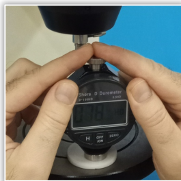
Figure 6. The device for measuring the hardness of ABS parts
