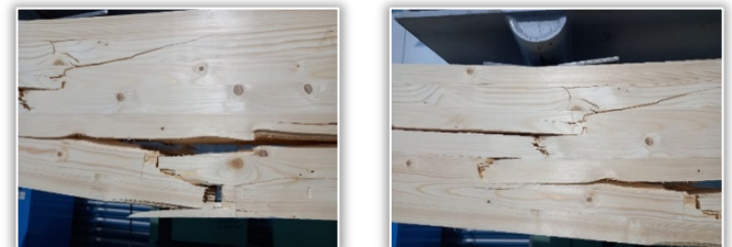
Figure 6. Failure patterns of the tested specimen Type 3 (SikaDur 330 + Sika Wrap 23°C)
