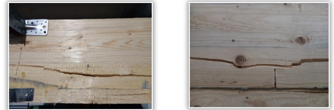
Figure 5. Failure patterns of the tested specimen Type 2 (SikaDur 330 + Sika Wrap 23°C)
