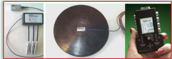
Figure 3. a) Accelerometer ACL 300, b) Single ACL and mounted on the pad, c) Data log device.
