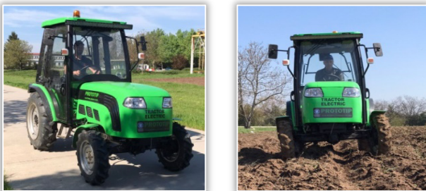
Figure 2 – Description of the protocol for the experimental tests carried out on the 2 types of roads at constant speed of 5 km/h: a) straight terrain; b) arable land.
