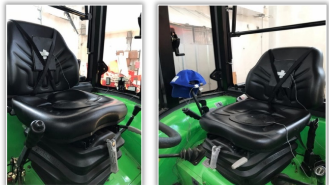
Figure 4 – Mounting of tri-axial accelerometers on the surface of the tractor seat and on the seat back
