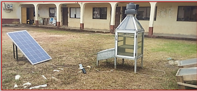
Figure 3: A pictorial view of an active solar dryer used for the experiment
