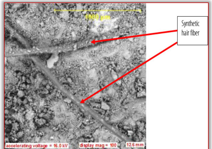
Figure 6: SEM micrograph of concrete with 2% addition of SHF
