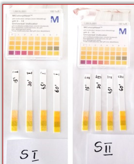
Figure 4 – pH in solution for Sample I—with molasses and Sample II without molasses
