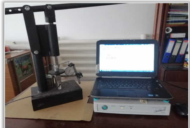
Figure 3 – Test equipment for determining the compressive strength of granular fertilizer material based on biosolids
