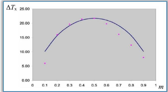
Figure3. Comparison of the computational data with experimental data Calculation —, Experiment •••• (T=293K, G=0,0032kg/s, P=168KPa)
