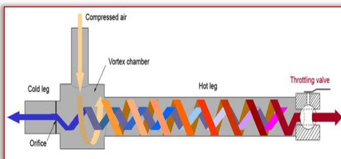
Figure1. Separation of a compressed gas into a hot stream and a cold stream
