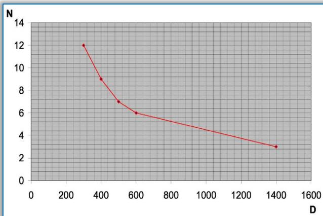
Figure.2. Changes of the number of macroscopic vortexes as compared to diameter of vortex tube for the (calculation) devices
