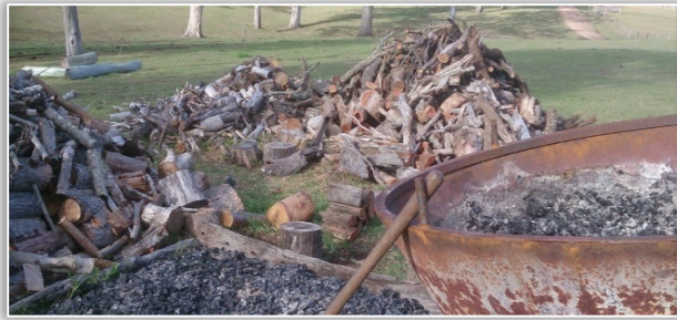
Figure 3 – a) and b) – simple small-scale production system in open field: a) Biomass burning; b) Biochar obtained after burning
