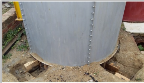
Figure 6 – BKI-type ovens, assembly view ( https://biocharkilns.com/biochar/ )
