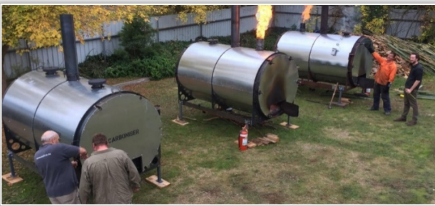
Figure 4 – Fixed unit for biochar production – Carboniser
