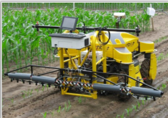
Figure 7 – Autonomous robot for protecting agricultural crops designed at the University of Aarhus, Denmark (Grulová et al. 2020)
