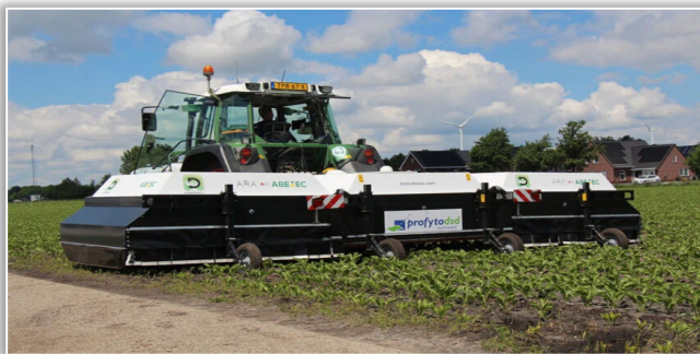
Figure 11 – ARA – EcoRobotix's plant sprayer that uses artificial intelligence, computer vision and computer systems to detect and selectively spray weeds with a micro-dose of herbicide | © Ecorobotix ( https://optics.org/news/12/3/52 )
