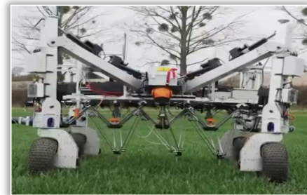
Figure 16 – Modern agricultural systems named Tom, Dick and Harry, developed by the Small Robot Company
