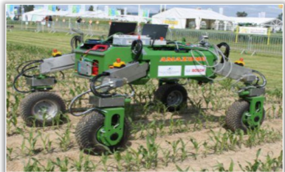
Figure 9 – Autonomous robot for agriculture designed at the University of Osnabrück in collaboration with Amazone and Bosch (Tilneac et al. 2012)
