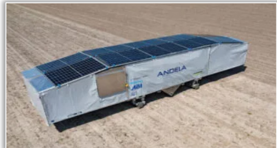
Figure 12 – The autonomous weeding robot is 9 meters wide and has 12 weeding units. On the roof are solar panels for electric motors.
