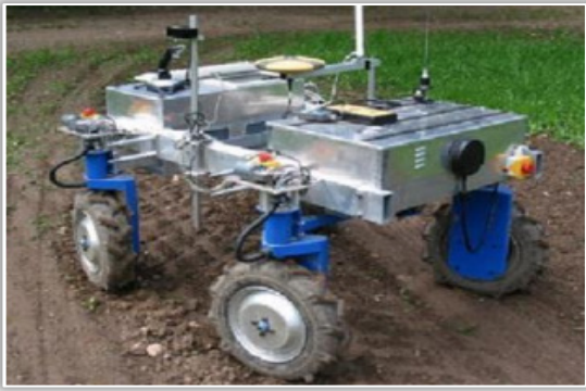
Figure 5 – Autonomous weed control robot designed at the Danish Institute of Agricultural Sciences, Denmark ( https://optics.org/news/12/3/52 )
