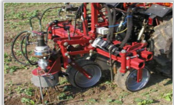
Figure 3 – “Querhacke” cycloidal harrow designed at the University of Osnabrück, Germany (Gruľová et al. 2020)
