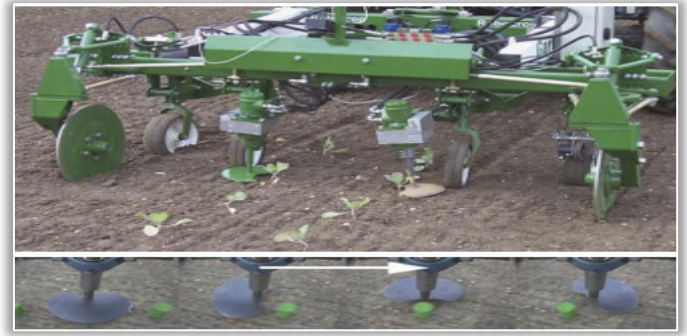
Figure 2 – Rotary disc provided with a section to protect cultivated plants ( https://optics.org/news/12/3/52 )
