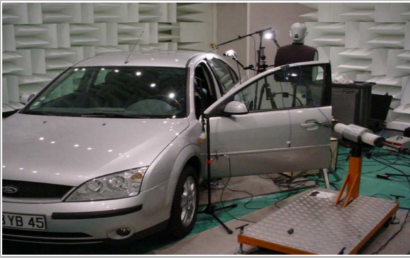
Figure 2. Measurement of the sound of closing car doors
