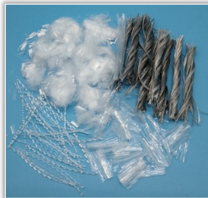
Figure 4. Plastic as microfibers (used for reinforcement)
