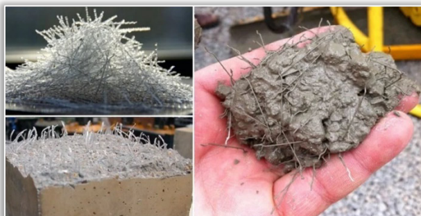
Figure 5. Fibre reinforcement with plastics in concrete
