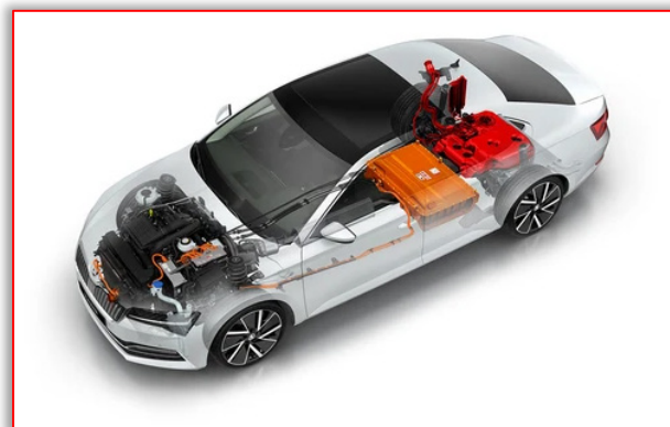
Figure 5. The drive system of the Škoda Superb III. [21]
