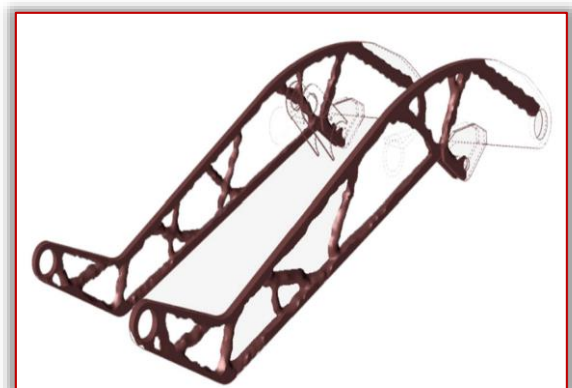
Figure 8. Topological optimization using the Altair Inspire [Dolmatov S. et. al. (2024)]
