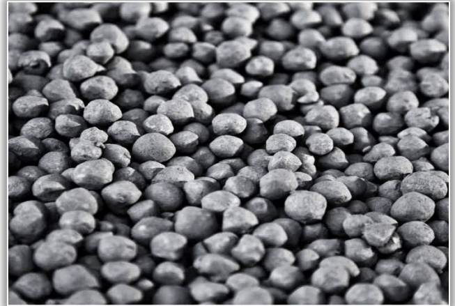
Figure 3. Pellets from fine ferrous wastes
