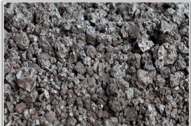
Figure 4. Sinter from fine ferrous wastes
