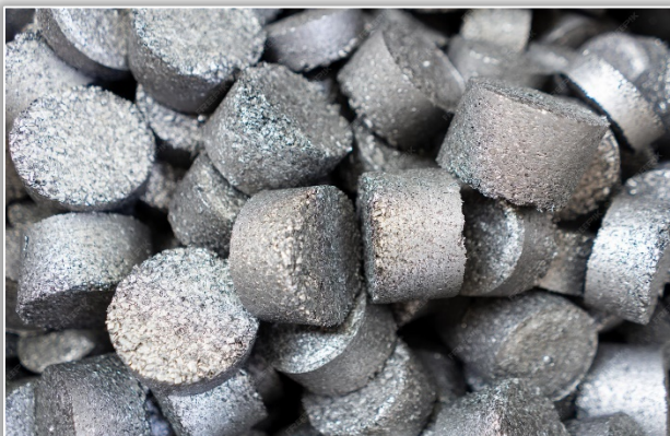
Figure 2. Briquettes from fine ferrous wastes
