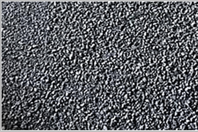
Figure 5. Granules from fine ferrous wastes
