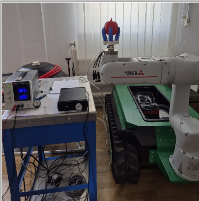
Figure 1. Gripper mounting on the test stand
