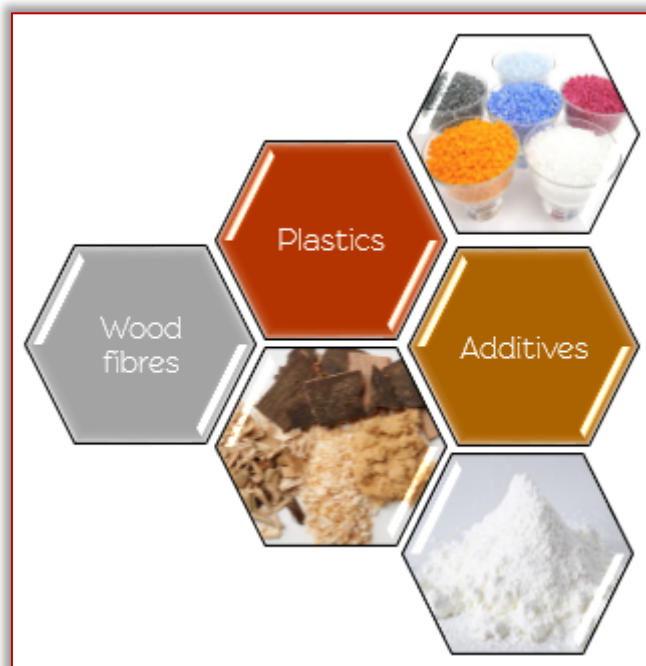
Figure 2. The components of WPC
