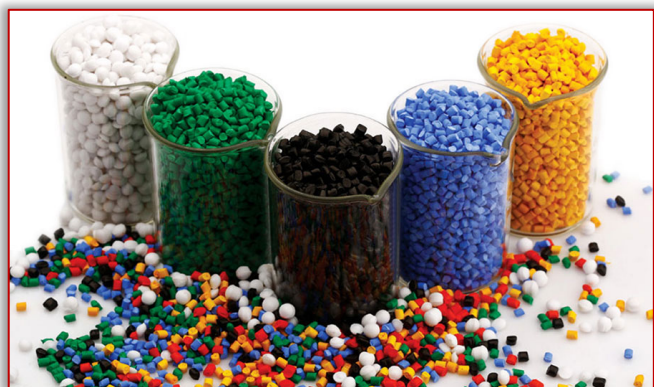
Figure 4. The plastic component in WPCs
