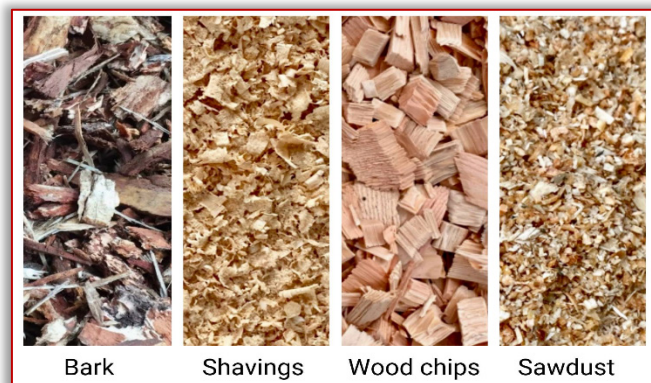
Figure 3. The wood components in WPCs
