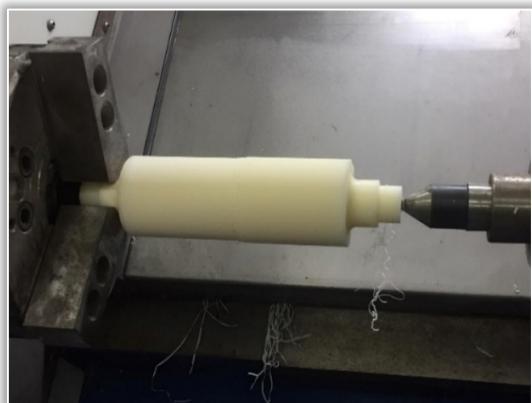
Figure 5. CNC Turning of the Roller Component
