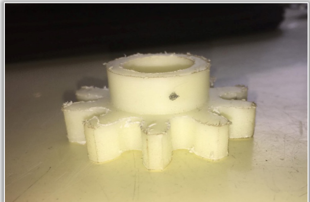
Figure 8. The experimental machining and final product of the spur gear
