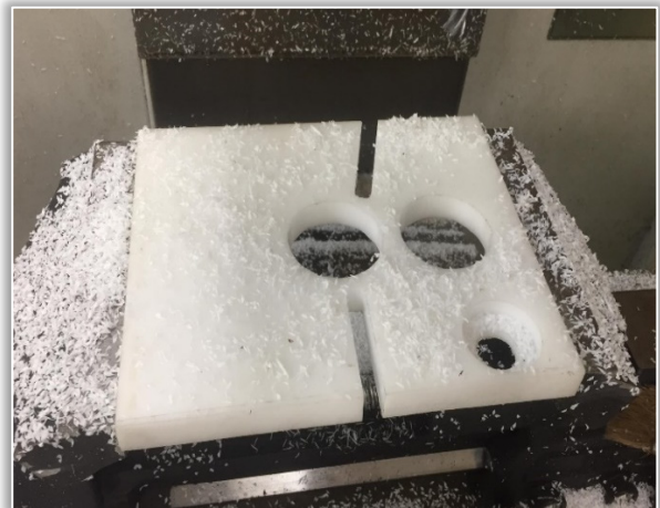
Figure 3. CNC milling of the side plate made from POM engineering plastic
