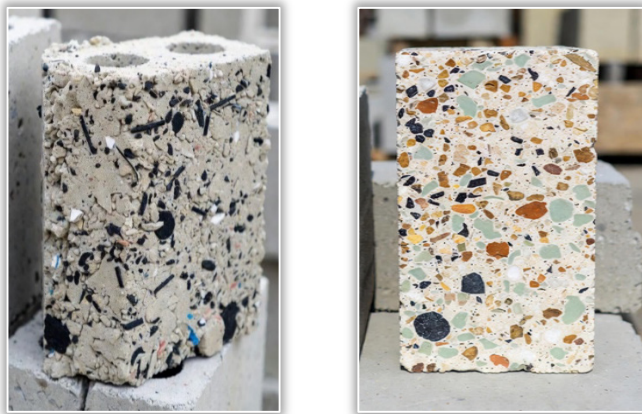
Figure 1. Eco-friendly concrete blocks produced with recycled concrete aggregates, waste PET fibers, crumb rubber, recycled glass cullet, and supplementary cementitious materials
