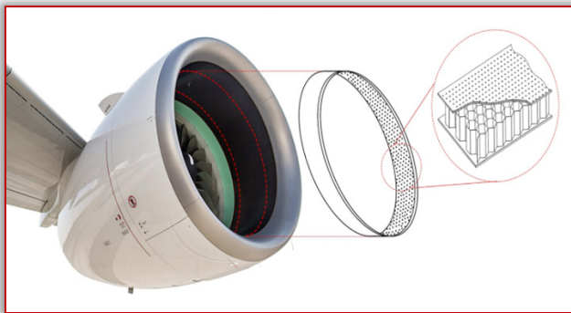
Figure 1 – typical structure for an acoustic liner of a turbofan engine [11]
