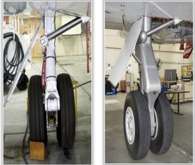
Figure 4 – landing gear (a – without porous fairing; b – porous fairing mounted in front of the rod) [18]
