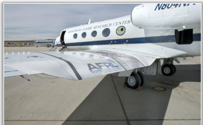
Figure 5 – ACTE wing flap mounted on a GIII airplane [20]
