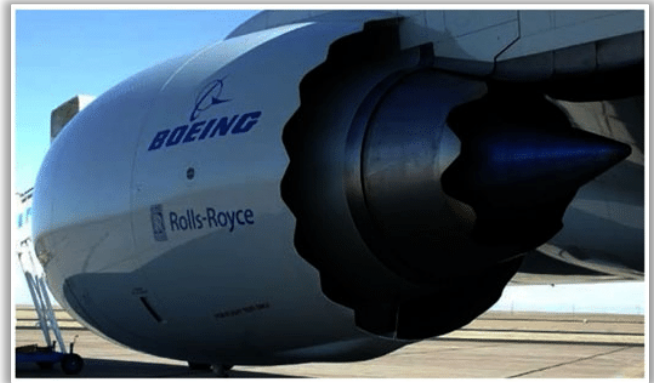
Figure 2 – chevron nozzles on Boeing 787 aircraft [13]
