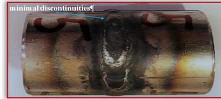
Figure 1 – Representative weld discontinuities associated with different welding technologies used in hygienic applications [12]
