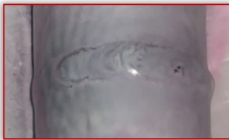
Figure 2. Surface-breaking discontinuities identified by penetrant testing in MAG and TIG welded specimens [12]; a) MAG welding, b) TIG welding
