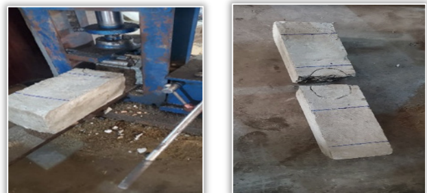
Failure mode of the control beam (A)
