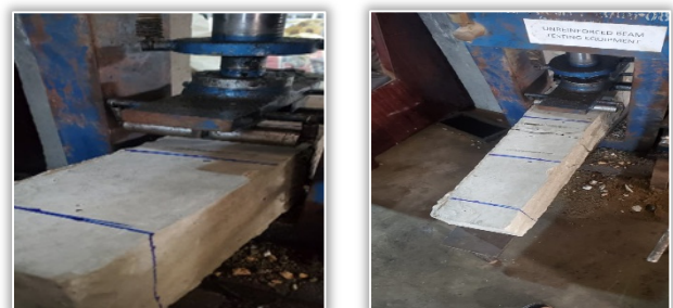
Failure mode of fibre reinforced beam (B)
