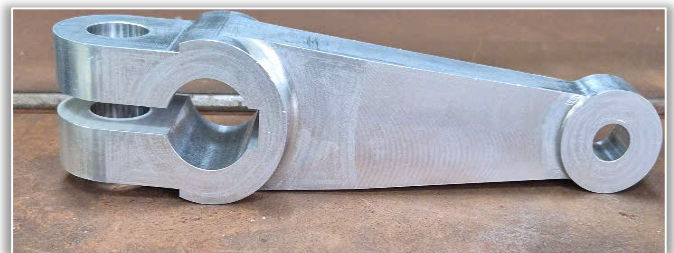
Figure 6. The completed mechanical linkage arm
