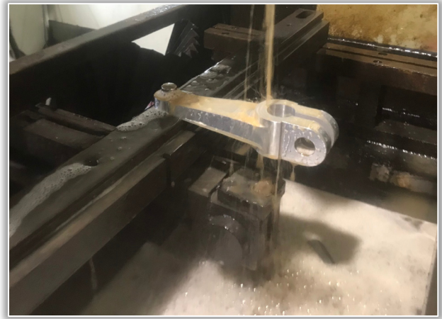
Figure 5. The keyway cutting process
