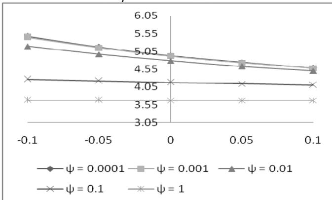
Figure 13. Variation of Load carrying capacity with respect to  $\bar{\beta}$  and  $\bar{\psi}$
