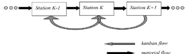
Fig. 1. Mechanism of the material and message flow in a Pull-type manufacturing system [3]
