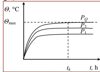
Fig.1. Graphical review of heating gear reducers depending on the input power (where  $t$  - time of heating,  $t_k$  - critical time when maximum permissible temperature is achieved ( $\Theta_{max}$ ),  $\Theta$  - temperature of the gearbox housing,  $P$  - input power of gearbox)
