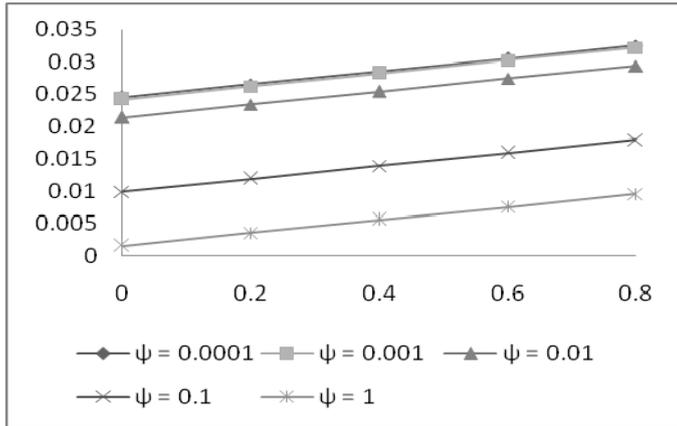
Figure 6. Variation of Load carrying capacity with respect to  $\bar{\alpha}$  and  $\psi$
