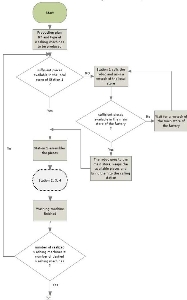
Fig. 2 : Flow-chart of the simplified process
