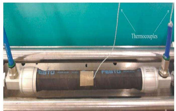
Figure 1 Muscle with two thermocouples
