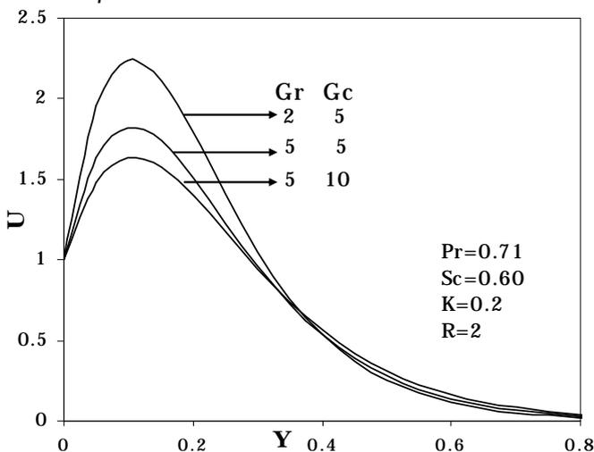
Figure 4. Velocity profiles for different values Gr, Gc
