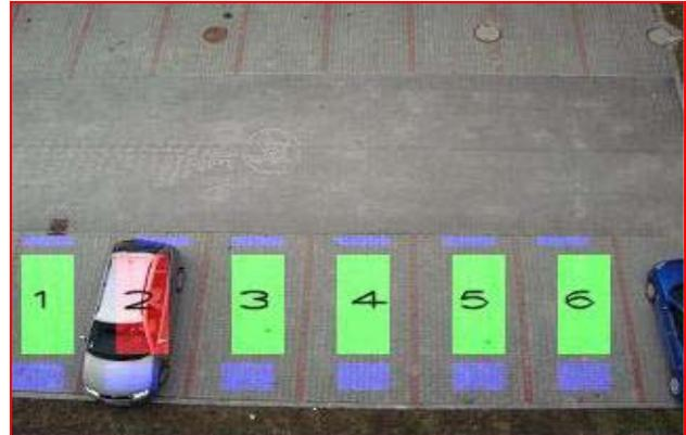
Figure 2. Example of ROI placement for parking places
