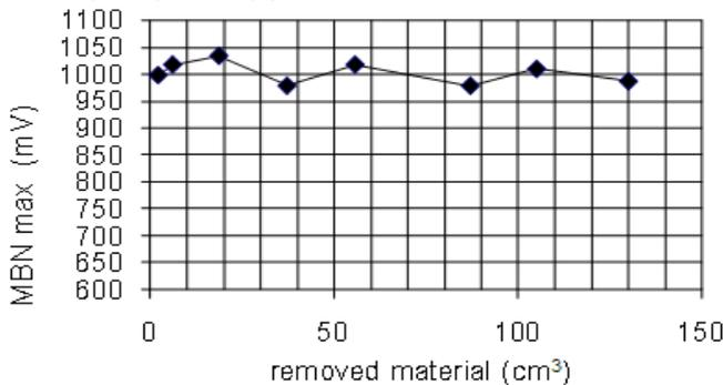
Figure 9. Influence of grinding wheel wear on amplitude of Barkhausen noise after turning
