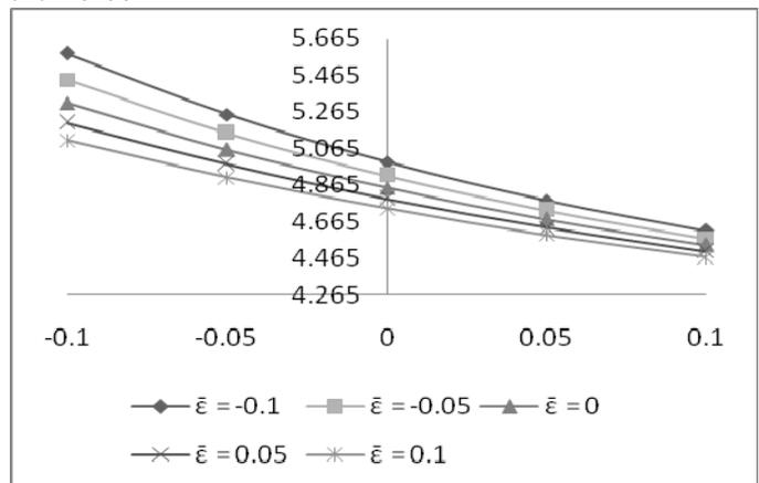
Figure 11. Variation of Load carrying capacity with respect to  $\bar{\alpha}$  and  $\bar{\epsilon}$
