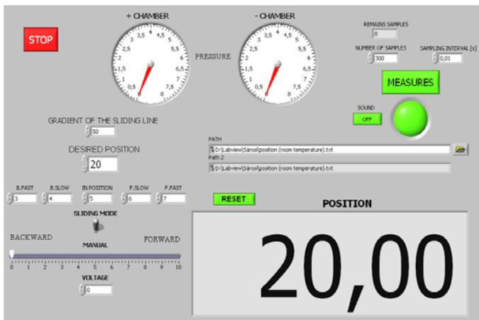
Figure 3 Front panel of LabVIEW program for positioning
