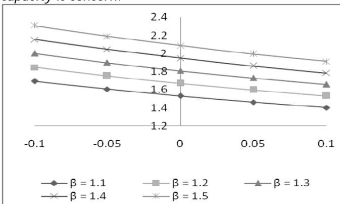
Figure 14. Variation of Load carrying capacity with respect to  $\bar{\sigma}$  and  $\bar{\psi}$
