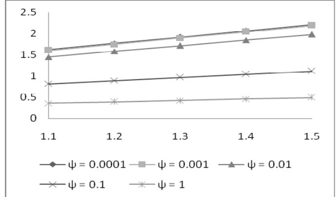
Figure 16. Variation of Load carrying capacity with respect to  $\bar{\sigma}$  and  $\bar{\psi}$
