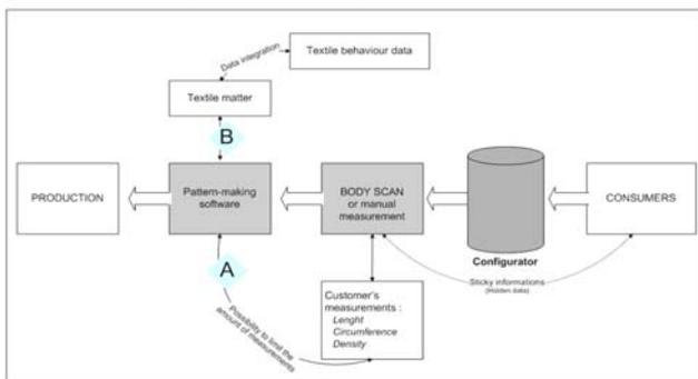
Fig. 1. Configuration for Clothing Mass Customization
