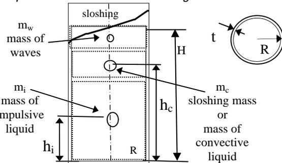
Figure 4. Seismic masses
