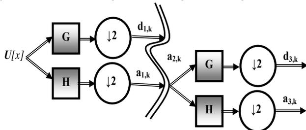
Figure 3 - Diagram of fast wavelet transformation  $m=3$  levels
