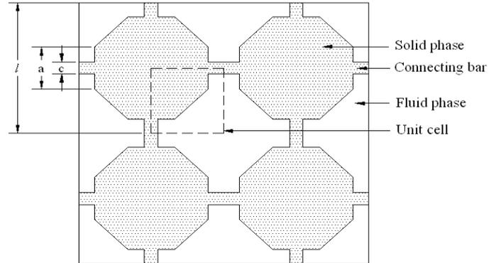
Fig.5. Two-dimensional spatially periodic two-phase system (Touching octagon cylinder)
