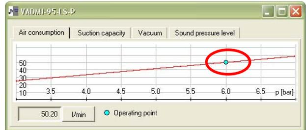
Figure 6 - Compressed air consumption at pressure level 6 bar
