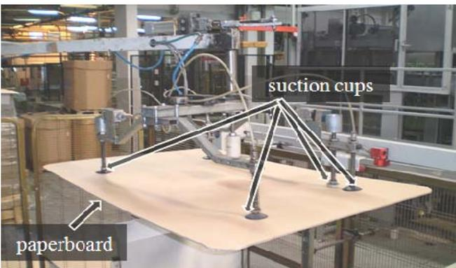
Figure 3 - Picking up the paperboard with suction cups
