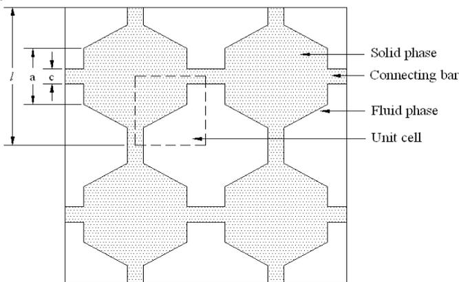
Fig.3. Two-dimensional spatially periodic two-phase system (Touching hexagon cylinder)
