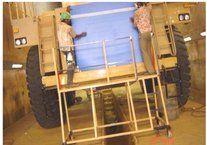
Figure 9. Masking with safety trolley - operator risk eliminated
