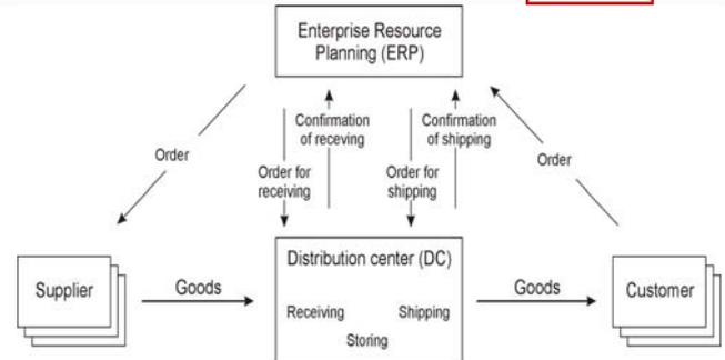
Figure 3 - Information flow in the supply network
