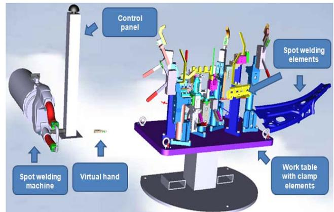
Figure 5 - Virtual work stand for spot welding
