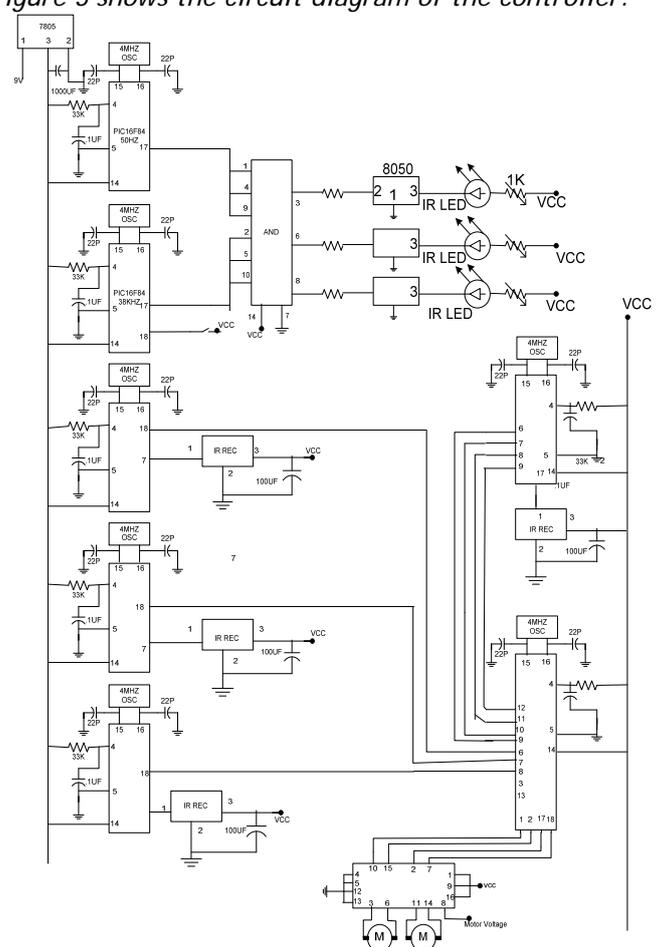
Figure 3: Circuit diagram of the designed controller
