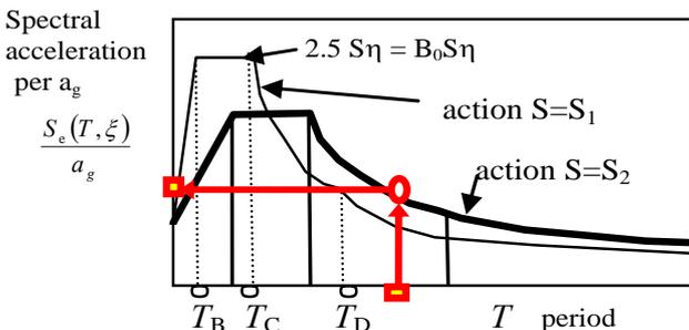
Figure 3. Spectral horizontal acceleration per ground acceleration vs. period of eigenvibration of the structure
