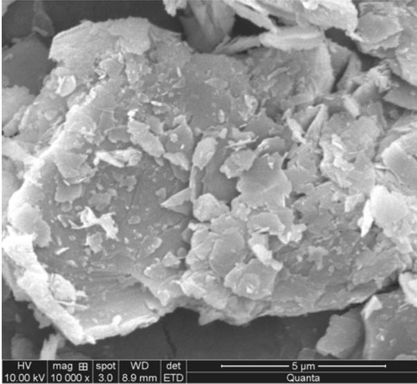
Fig 3 SEM Photo of Kaolinite at 25°C
