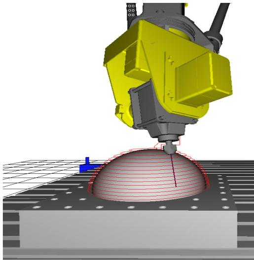
Figure 6 - CL DATA application for 5-axis milling
