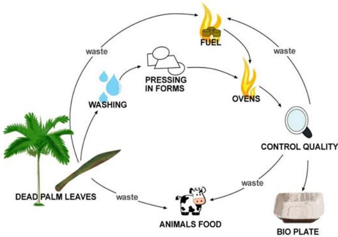
Figure 4 - Simplified systemic BioPlate production process
