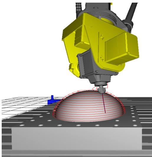
Figure 6 - CL DATA application for 5-axis milling
