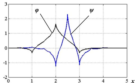
Figure 2 - The basic functions of wavelet Coiflet 1 ‘coif1’
