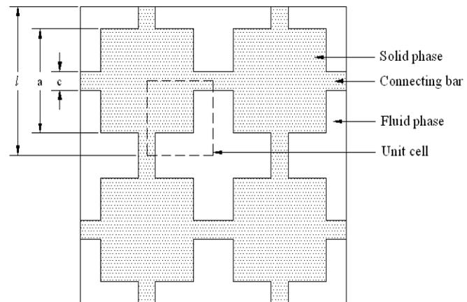
Fig. 1. Two-dimensional spatially periodic two-phase system (Touching square cylinder)
