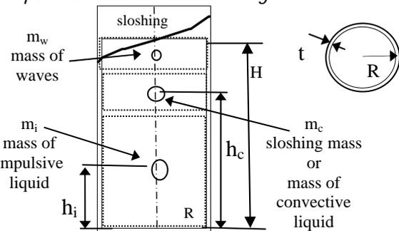
Figure 4. Seismic masses
