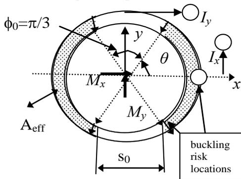
Figure 9. Skirt cross section at opening
