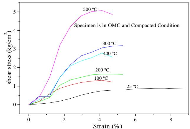
Figure 2. Shear stress Vs strain in Kaolinite clay
