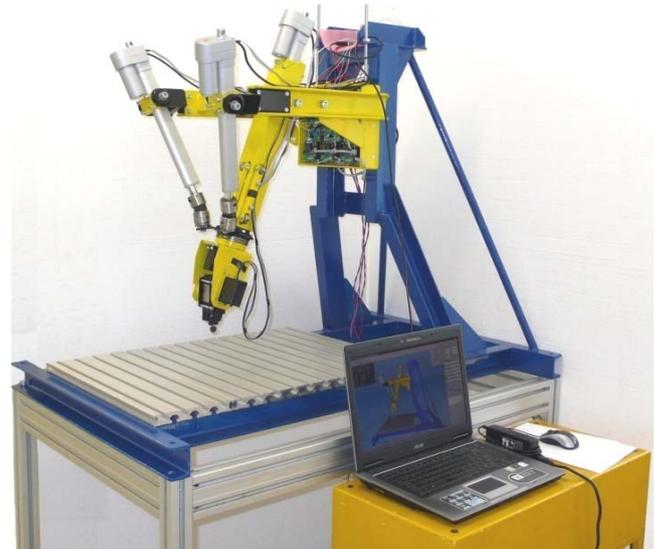
Figure 9 - Small-scale CNC machine tool builds on trivariant hybrid kinematic structure
