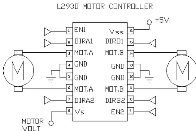
Figure 2. Pin configuration of L293D motor driver IC
