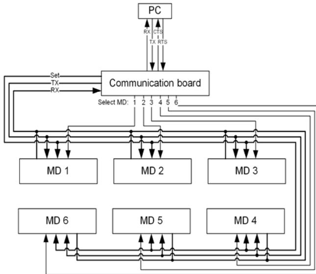
Figure 8 - Communication interfaces in control system
