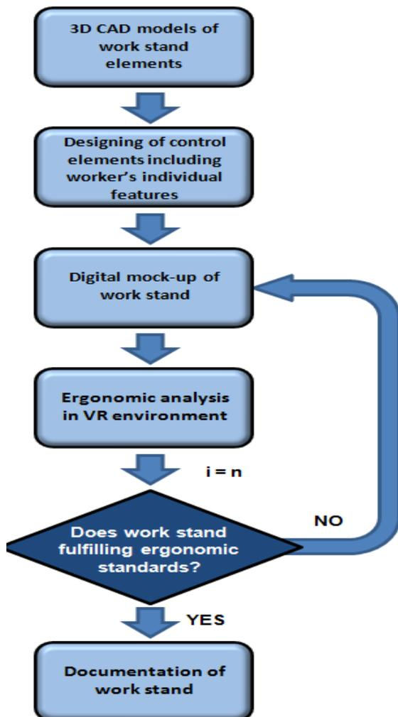
Figure 4 - Work stand design process using VR system
