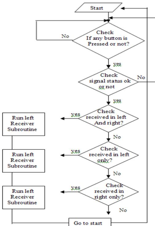
Figure 4: Flow chart for obstacle detection system
