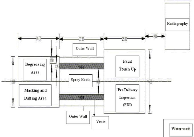
Figure 2. Layout of the assembly line paint shop
