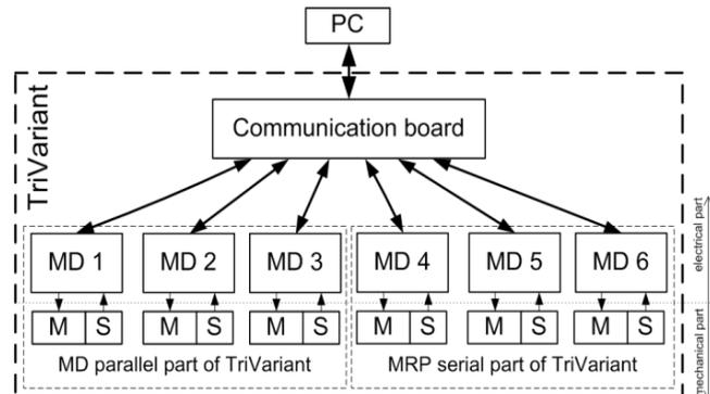
Figure 7 - Block diagram of designed control system
