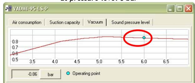
Figure 7 - Vacuum level at pressure level 6 bar
