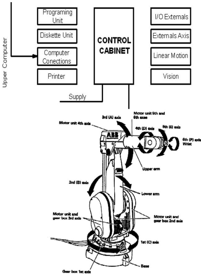
Fig. 1 main ABB IRB 2000 hardware and software components
