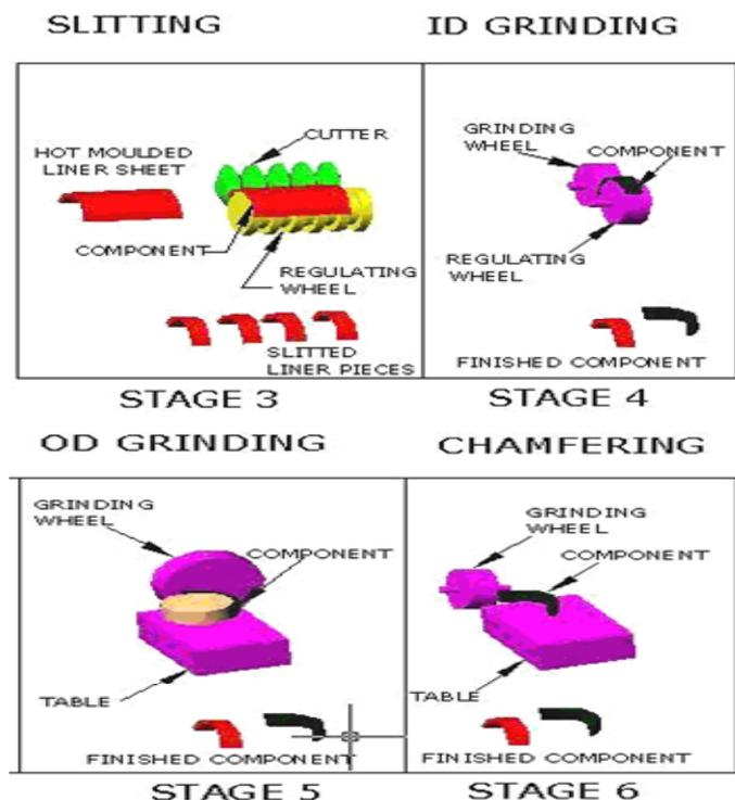
Figure 1. Machining stages of brake liners
