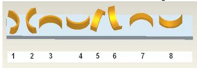
Figure 3. Resting orientations of brakeliner
