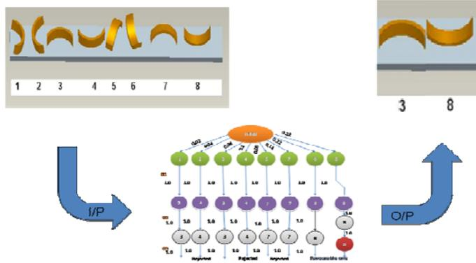
Figure 7. Markov model for trap I (Probability for Preferred orientation = 0.54)
