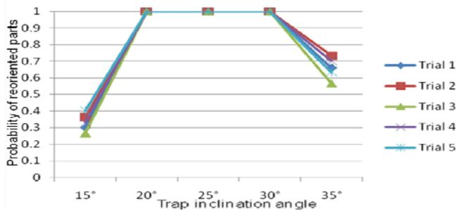
Figure 14. Effect of trap inclination angle on successful orientation of parts
