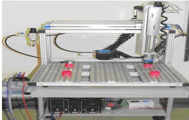
Fig. 2 Real construction „Pick and Place“ manipulator controlled by PLC
