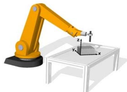
Figure 5. Workpiece coordinates
