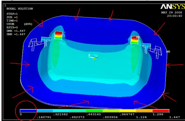
Figure 6. Edges experiencing no deformation
