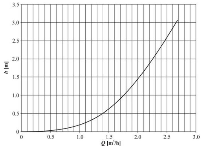
Figure 5. The performance curve of filter nozzle model RV001/A for the filtration process
