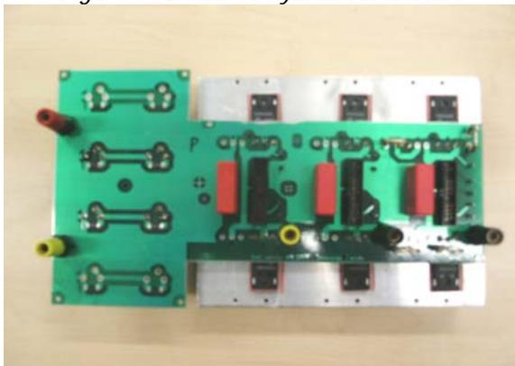
Figure 10. Prototype of VSI with classical IGBTs
