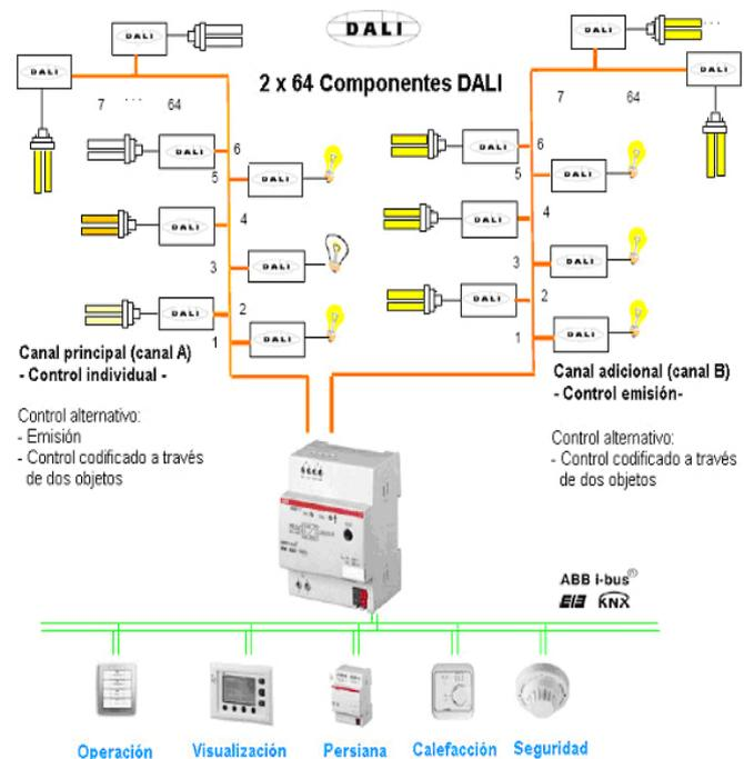
Figure 3. The KNX and DALI network
