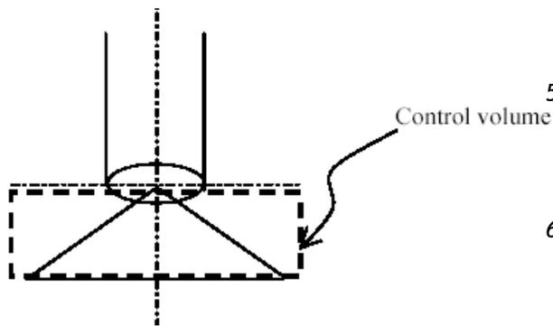
Figure1. Control volume of spray with conical pattern
