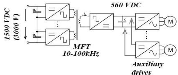
Figure 12. Principal scheme of auxiliary drives traction converter
