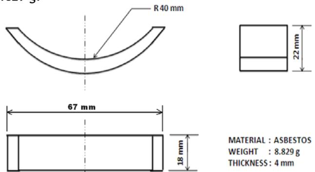
Figure 2. Brake liner
