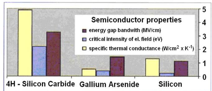
Figure 1. Comparison of individual semiconductor features [3]
