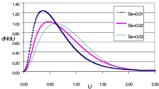
Figure 9 - Curves of the dimensionless diameter distribution of the sprayed droplets at the distance of 10cm from the nozzle versus momentum source term
