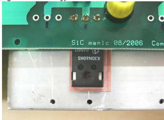
Figure 11. Detail of VSI with classical device
