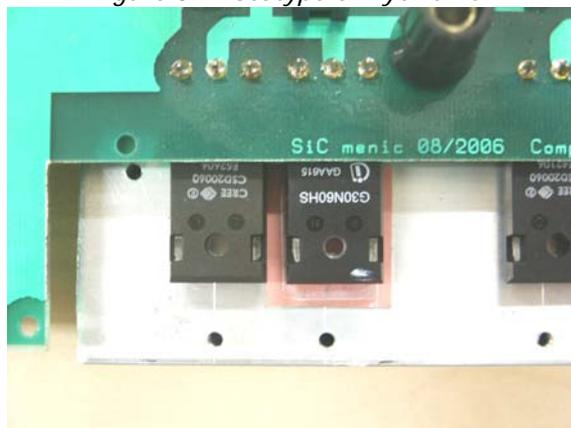
Figure 9. Detail of hybrid VSI devices
