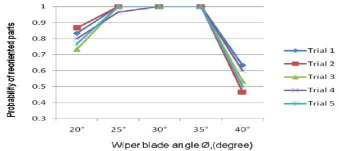
Figure 13. Effect of wiper blade angle on successful orientation of parts
