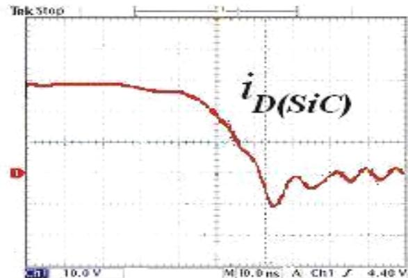
Figure 5. Current waveform of the SiC Schottky diode (produced by CREE as shown in Fig. 9)
