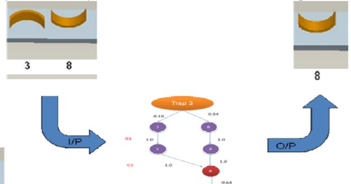
Figure 9. Markov model for trap II (Probability for Preferred orientation = 0.64)
