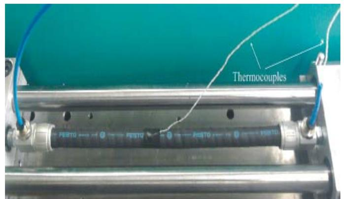
Figure 1. Muscle with two thermocouples
