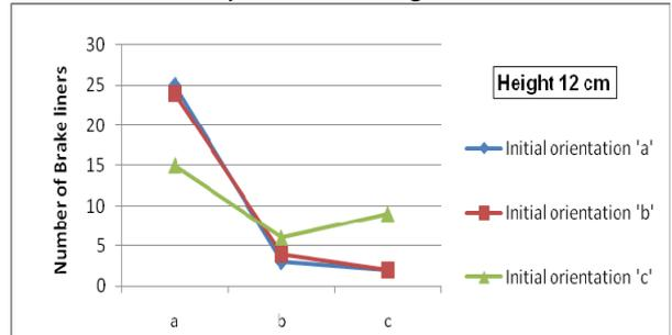
Figure 5(b) Effect of initial orientation when dropped from 12 cm height
