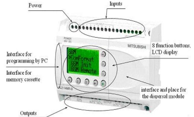
Fig. 6 Programming machine Mishubishi Alpha
