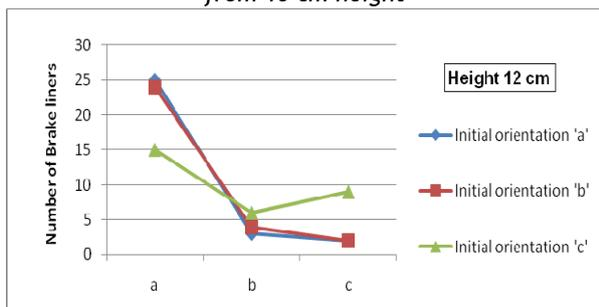
Figure 5(b) Effect of initial orientation when dropped from 12 cm height
