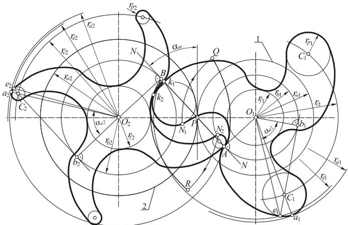
Figure 3. Asymmetric involute-lantern meshing  $z_1 = 3, z_2 = 4$
