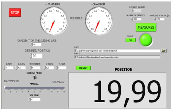
Figure 3 Front panel of LabVIEW program for positioning
