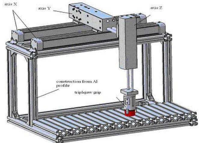
Fig. 3 Three-axis pneumatic „Pick and Place“ workstation design
