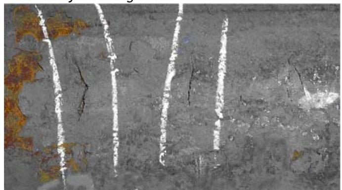
Fig. 6. Transverse cracks
