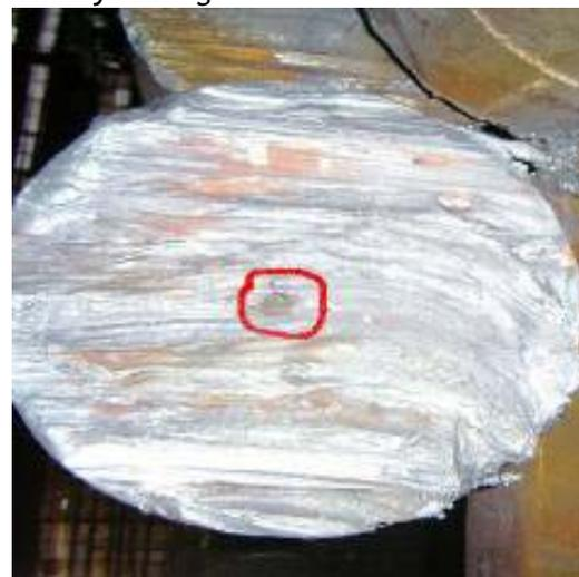
Fig. 12. Shrinkage cavity
