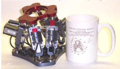
Figure 3.14 Parallel micro robot [52]
