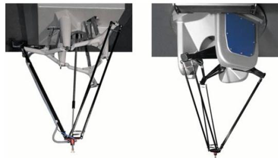
Figure 3.17 Two of the three Delta robot models offered by SIG Pack Systems, C33 and CE33 (courtesy of SIG Pack Systems-now Bosch Packaging Technology division)
