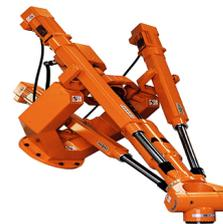
Figure 3.21 Parallel kinematic robot Tricept IRB 940 [50] The initial challenge for this system was that it required computer power that was unavailable at the time. Karl-Erik Neumann, the inventor of the Tricept robot, explains: "There was no control system to run the machine until 1992 when the company Comau Pico launched the first multiprocessor controller. That, and open architecture, made it so we could adapt its complex kinematics [10].
