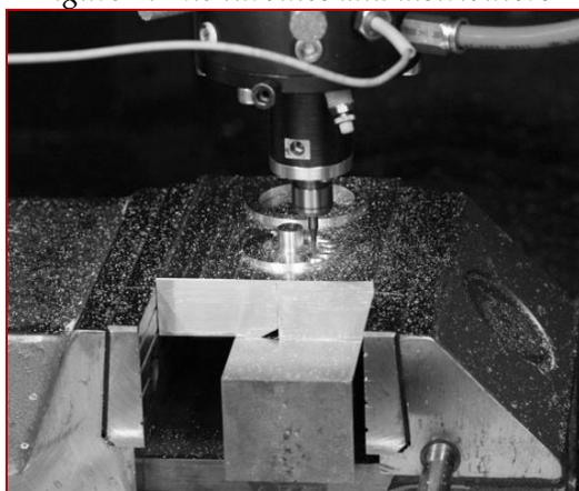
Figure 5: Production of radial air turbine and distributor
