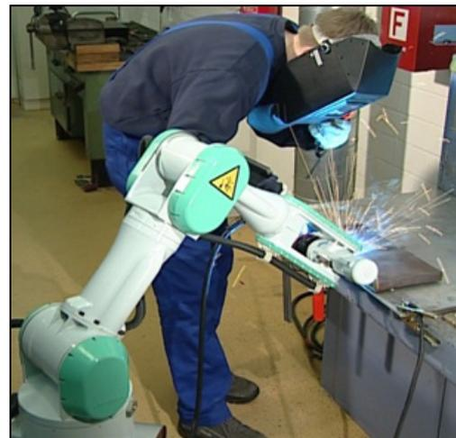
Figure 3. Two workers collaborating and working together with traditional six-axis robots [6] [7].
