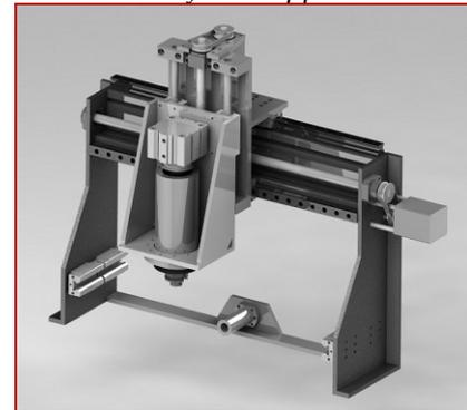
Figure 3. The module of the Y axis (gantry module)
