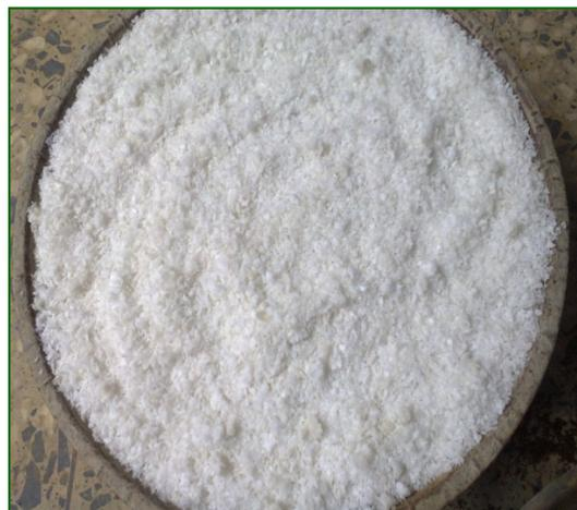
Figure 1: Recycled Polypropylene fibres
