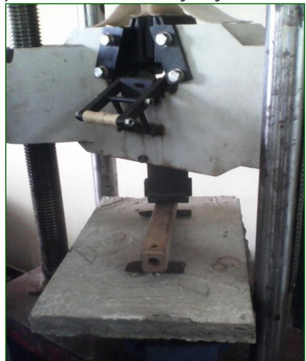
Figure 3: Slab specimen undergoing 3 points loading
