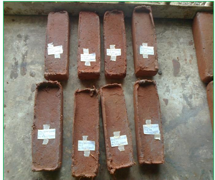
Figure 5. Composite samples prepared for flexural test
