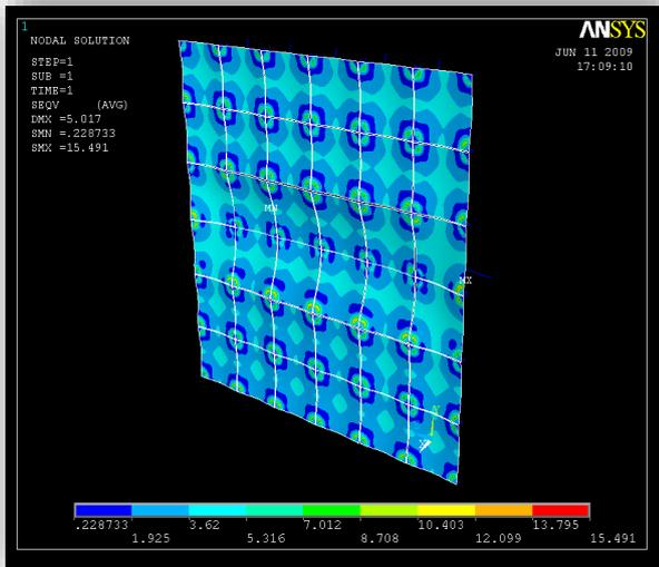
Figure 25. Stress distri. in panels\*(low. temp)
