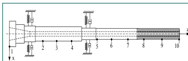
**Figure. 1.** Equivalent dynamic model of spindle with measurement points [4]
