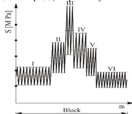
Figure 4. Load Spectra.
