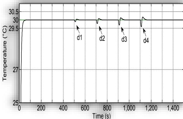
**Figure 5.** Enlarged view of temperature in flow tank under influence of disturbance (h+, t-)
