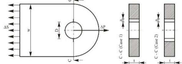
Figure 1. Geometry of the lug with through-the-thickness crack.
