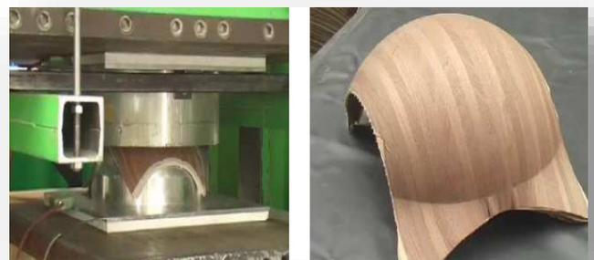
Figure 3. The process of making 3D plywood with male and female template [8]
