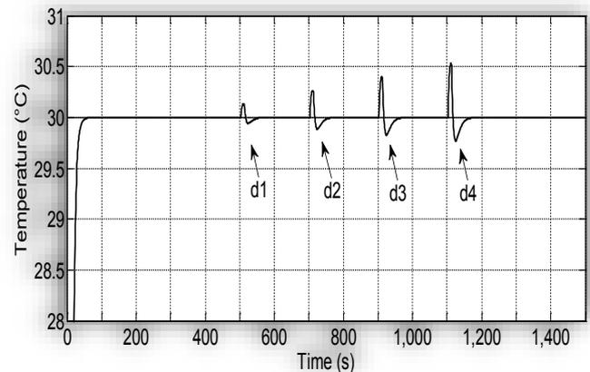
**Figure 7.** Enlarged view of temperature in flow tank under influence of disturbance (h-, t+)
