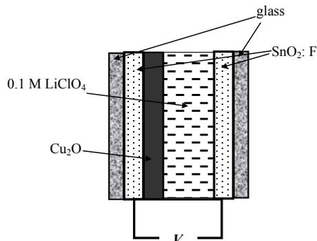
Figure 1. The cross-section of the so-designed ECTD
