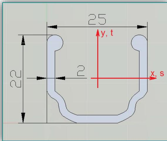
**Figure 1.** Cross section of the rim
