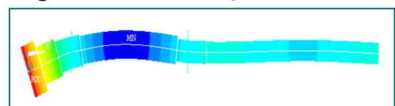
Figure 7. Third bending mode 1641 Hz
