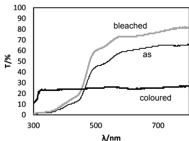
Figure 3. Transmittance spectra of the  $Cu_2O$  film.
