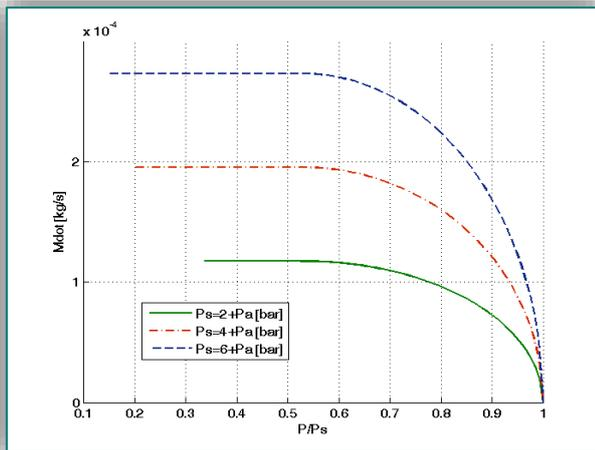
Figure 2. Mass flow rate through the fixed orifice
