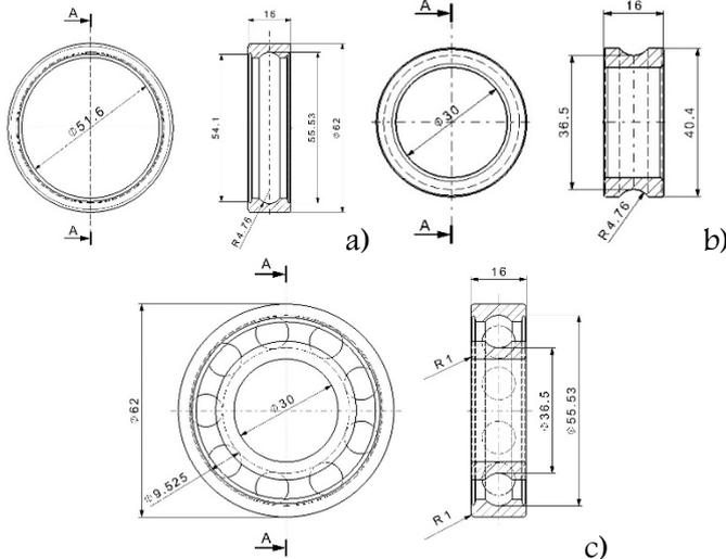
**Figure 1.** Geometrical size rolling ball bearing SKF 6206
