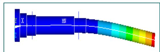
Figure 5. First bending mode 154,37 Hz
