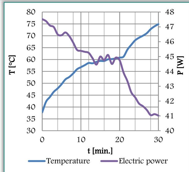
Figure 3. Relationship between the temperature and the power as a function of time
