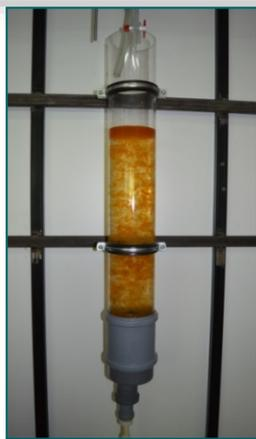
Figure 4. The reaction column for coagulation
