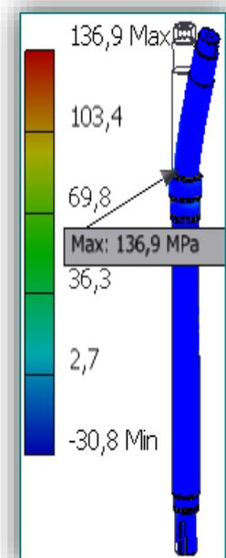
Figure 4. Distribution of the 1-st principle stresses
