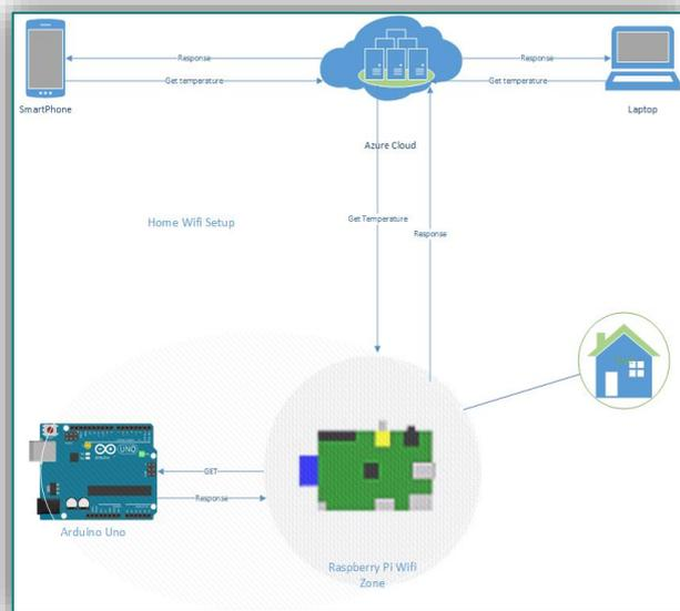
Figure 1. Network topology diagram of WoT devices
