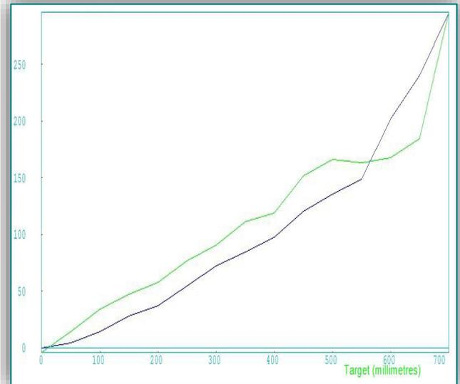
Figure 6. The measurement to determine the anomaly. From the resulting graph it was concluded that the measuring apparatus was not at fault, nor was the measurement procedure to blame for the anomaly, but rather the tolerances in the mechanism itself.
