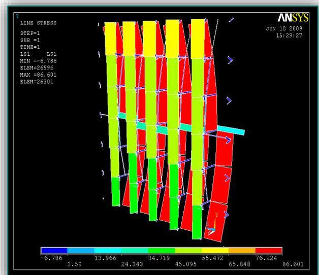
Figure 13. Stress in support structure
