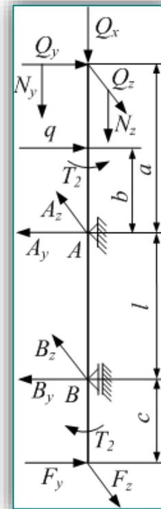
**Figure 1.** Scheme of loading of the cutting spindle
