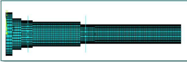
Figure 2. Discretized model of main spindle [4]
