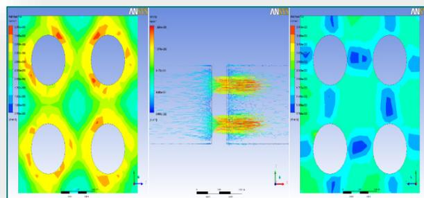
Figure 7. Numerical results for the Reynolds number 300 - air velocity of 1,24 m/s
