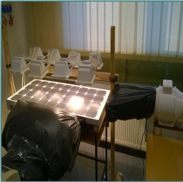
Figure 2. The illuminated PV module and the cooling system
