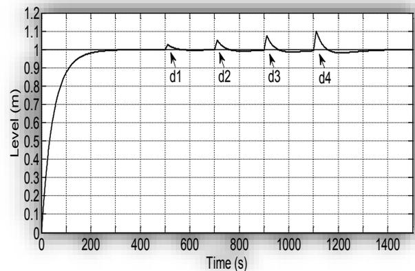
Figure 3. Level in flow tank under influence of disturbance (h+,t+)
