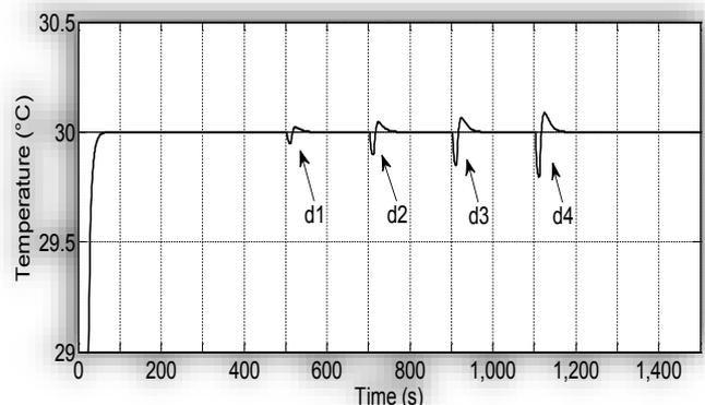
**Figure 8.** Enlarged view of temperature in flow tank under influence of disturbance (h-, t-)
