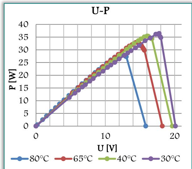
Figure 5. U-P characteristics in case of different temperatures
