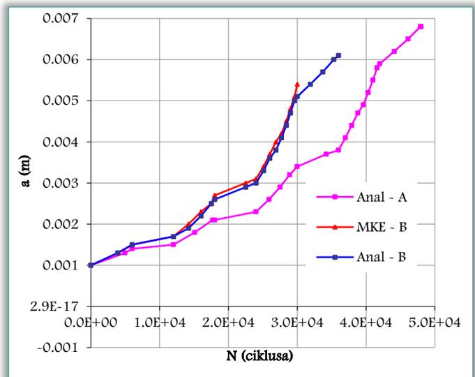
Figure 4. Surface crack growth under load spectra
