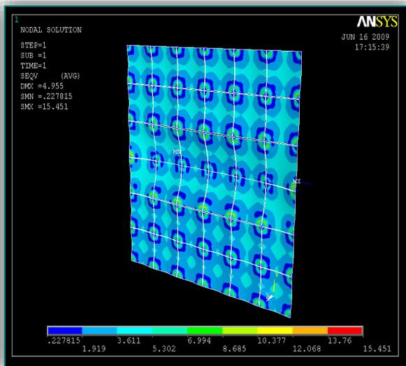
Figure 21. Stress distri. in panels\*(hig. temp)
