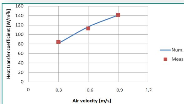
Figure 5. Comparison of the numerical model and experimental results for the overall heat transfer coefficient
