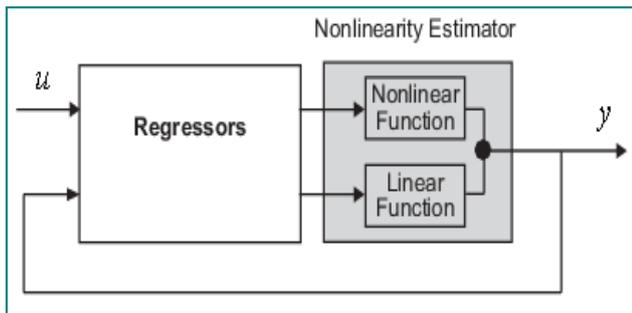
Figure 1. Structure of Nonlinear ARX Models.
