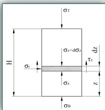
Figure 1: Stresses applied to a powder slice
