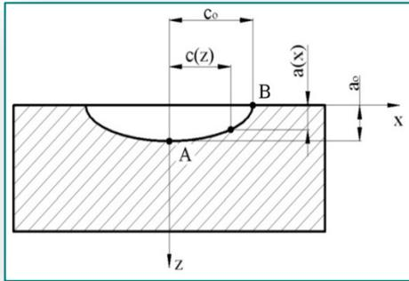
Figure 1. Surface crack idealization
