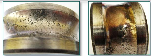
**Figure 3.** Fatigue wear (pitting) on the outer surface of the bearing inner track
