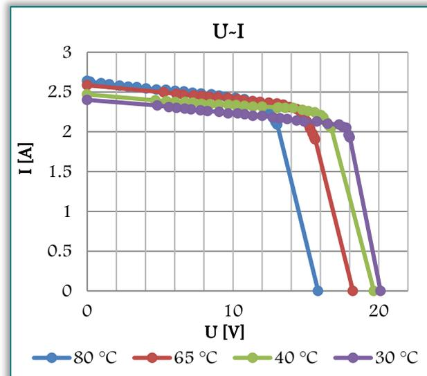
Figure 4. U-I characteristics in different temperatures
