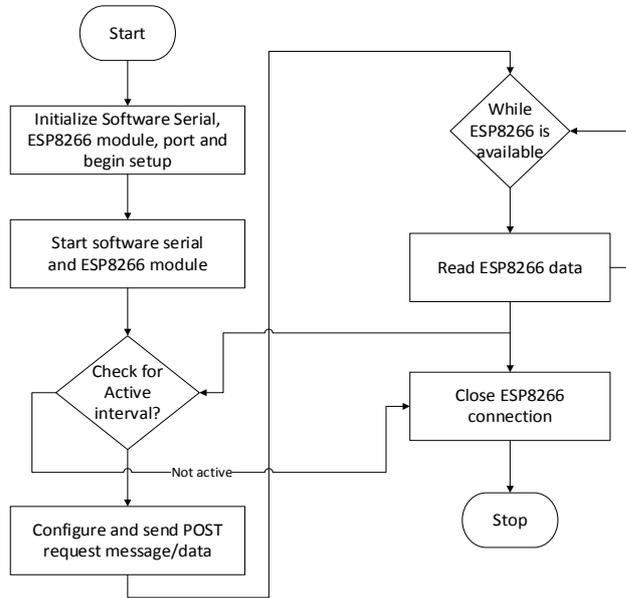
Figure 2. Arduino workflow
