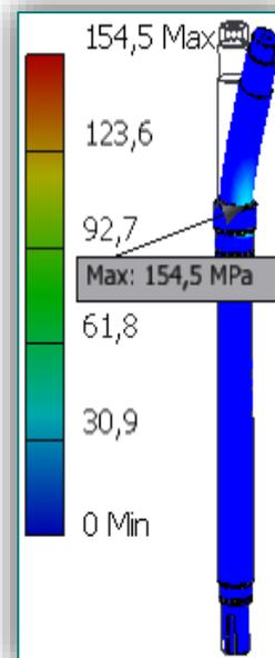
Figure 3. Distribution of the Von Mises stresses
