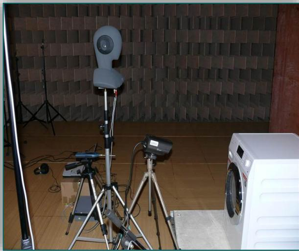
Figure 3. Binaural measurement of washing machine sound
