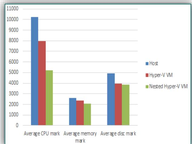
Figure 7. PassMark performance test compared overall results
