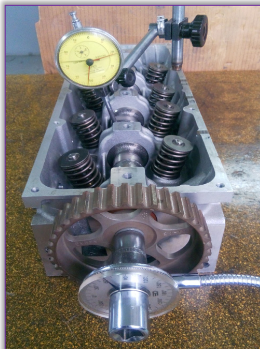
Figure 1: Determination of the dimensions of the cam
