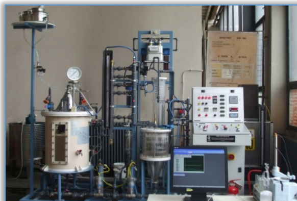
Fig. 1 - Small capacity plant for biogas production [8] The sample subjected to fermentation is heated by a heating element. Fermented mass is taken by means of a pump from the bottom or the top of the reactor, where it is further heated by resistance.
