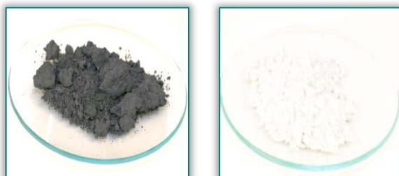
Figure 7. Graphite and Bentonite
