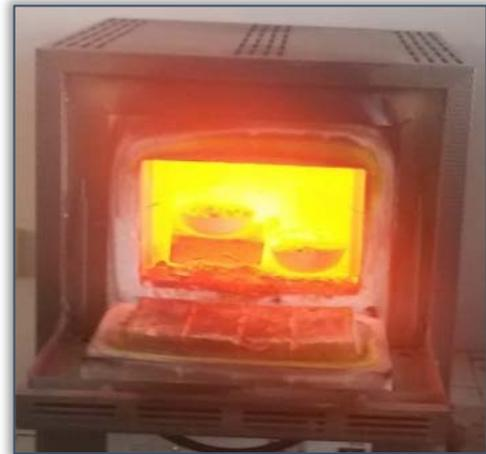
Figure 22. Pellets in the calcination oven
