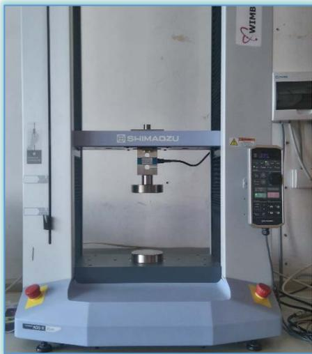
Figure 7. Testing machine with compressive module
