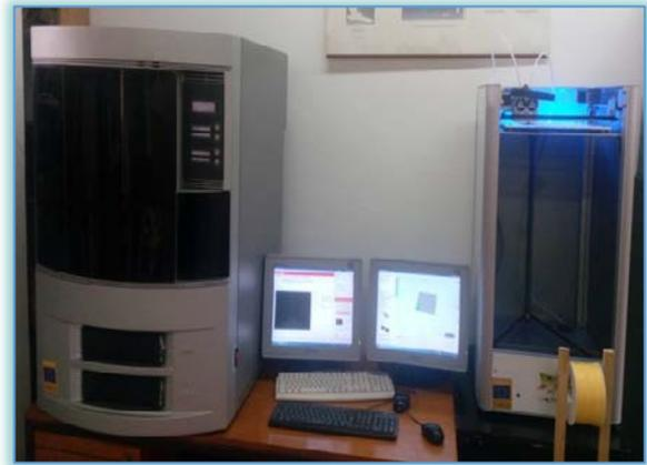
Figure 2. 3D printers: Dimension Elite (left) and LeapFrog Creatr XL (right)
