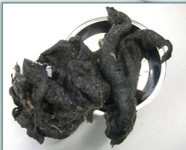
Figure 3. Composite materials after the homogenization [5]
