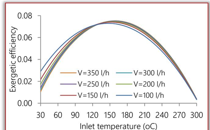
Figure 5. Exergetic efficiency for various flow rates
