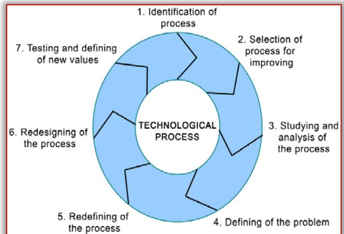
Figure 1. Stages in analysis of the technological process
