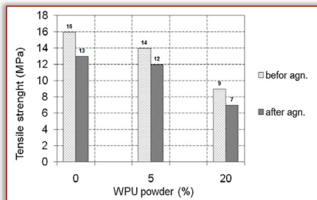
Figure 2. Results of tensile strength of rubber blends
