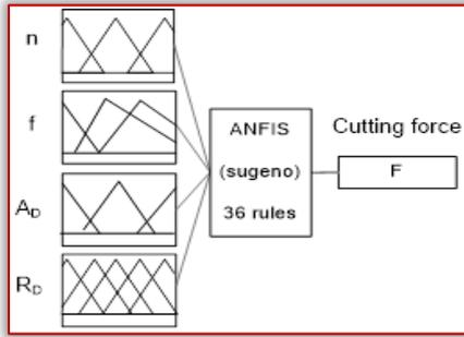
Figure 2 – Structure of ANFIS cutting force model
