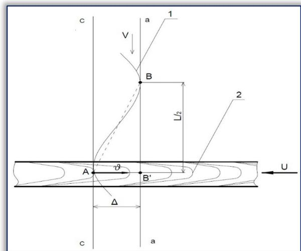
Figure 1: Scheme for determining the velocity of offset of a section of the band saw blade caused by its own axial run-out against the feed rate
