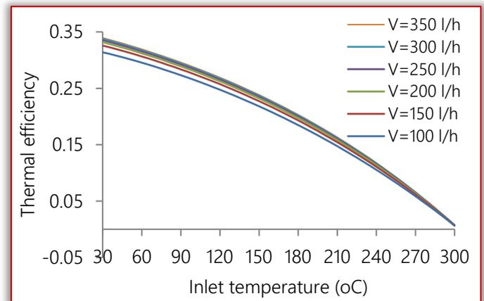
Figure 4. Thermal efficiency for various flow rates
