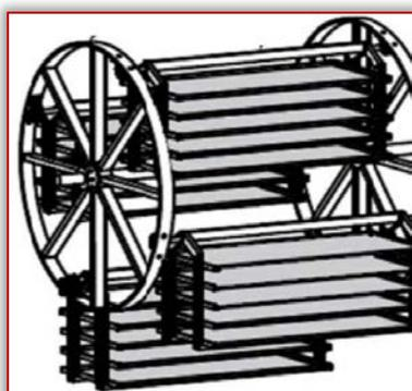
Figure 1. Representation of the rotary dryer interior
