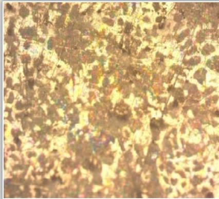
Figure 7: Eutectic cell of 12.5mm thickness x50
