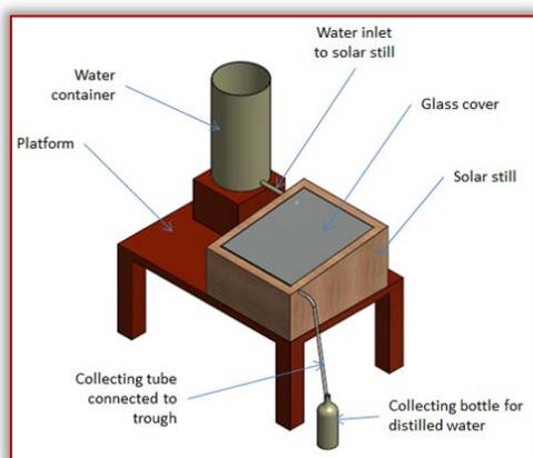
Figure 1. Experimental set-up of the solar water still.
