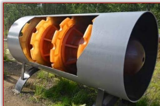
Figure 7. The appearance of the pipeline cleaner
