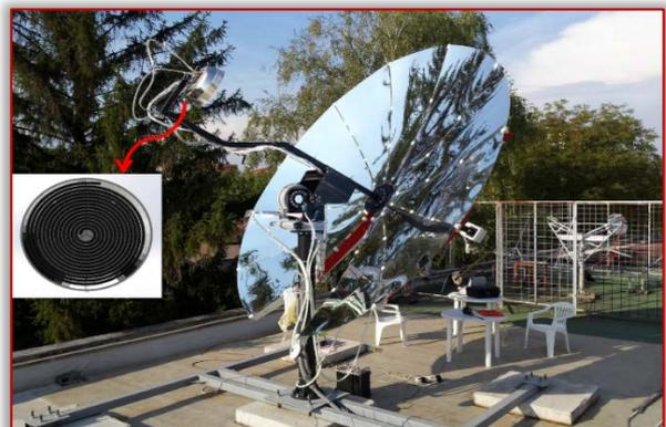
Figure 1. The examined solar dish collector
