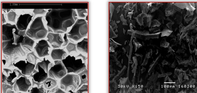
Figure 5. Appearance of PU before and after recycling
