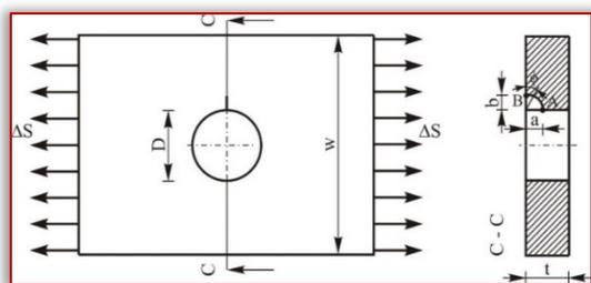
Figure 1. Geometry of the plate with quarter-elliptical corner crack emanating from a hole ( $a$  - depth direction,  $b$  - surface direction).
