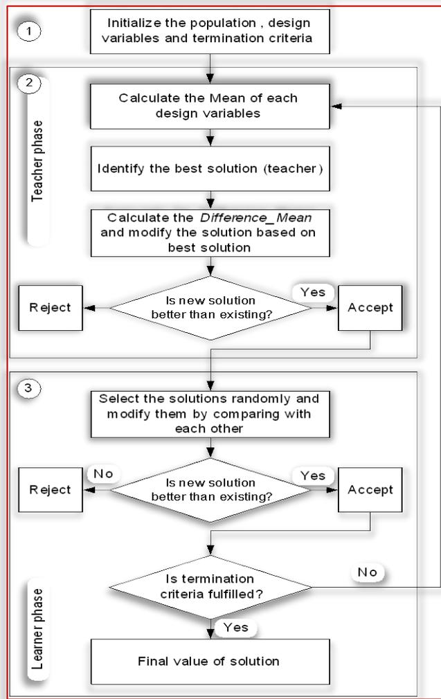
Figure 1 – The diagram of the TLBO algorithm
