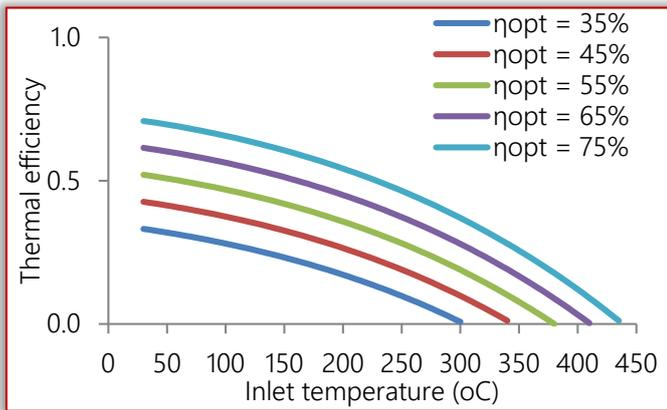
Figure 6. Thermal efficiency for various optical efficiencies
