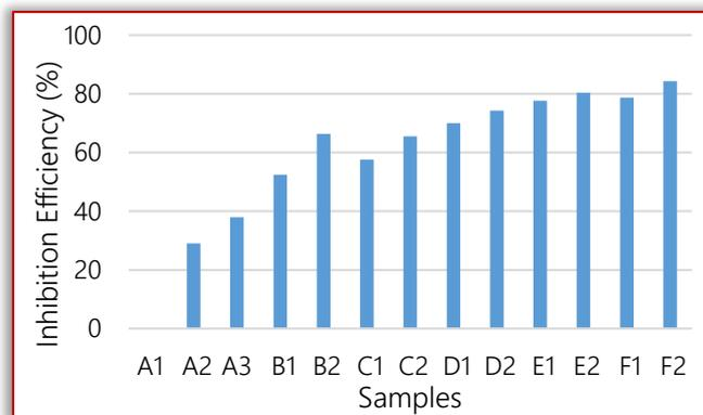
Figure 7: Dependence of Inhibition Efficiency on Sample Processing Condition for Mild Steel Painted in Red and White with 0-25% Zn Powder Addition
