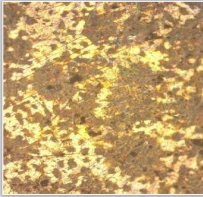
Figure 6: Eutectic cell 11.5 mm thickness x100
