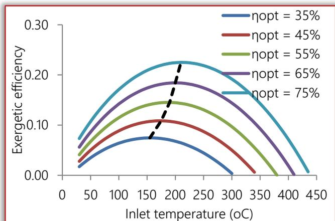
Figure 7. Exergetic efficiency for various optical efficiencies
