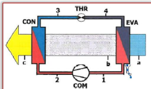
Figure 1. Principle of operation in a simplified heat pump dryer. After flowing through the evaporator and condenser of the heat pump the dry and warm air is ready to flow into the drying chamber in which the material, which is to be processed, is being placed. The simplified heat pump dryer has two separated loops with common heat exchangers. The drying air loop (abcd) contains the air cooler (EVA), heater
