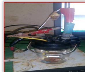
Plate 5: Electrochemical Measurement (TAFEL Polarization set-up)
