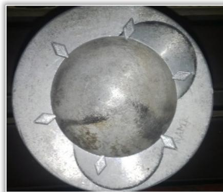
Figure 3.Top view of the Rhombus Grove Piston Crown
