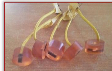
Plate 6: Coupons after TAFEL Polarization test
