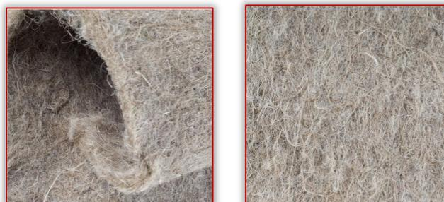
Figure 4. Bast fibers (flax, jute and hemp) solutions for non-woven mats
