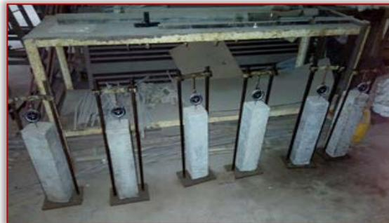
Figure 1: Specimens under shrinkage test
