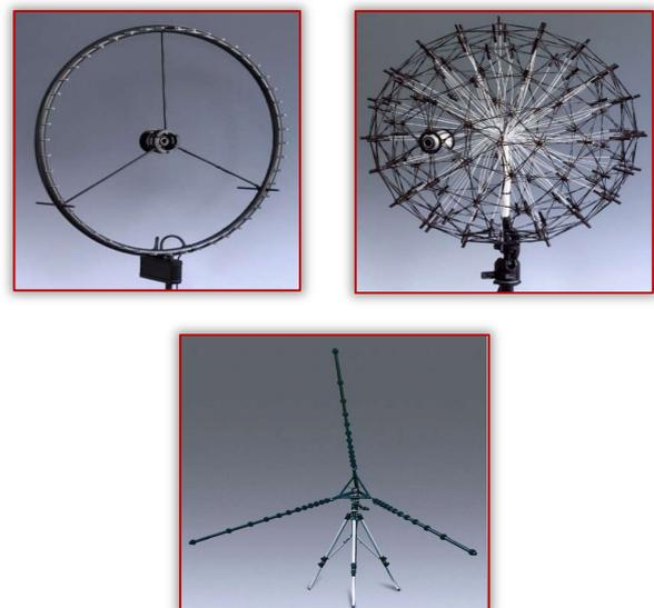
Figure 2. Microphone arrays of noise visualization tools [11]
