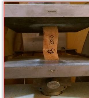
Figure 1: Failure mode of 200mm (Shear)
