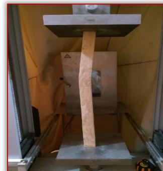
Figure 3: Failure mode of 200mm (Buckling)
