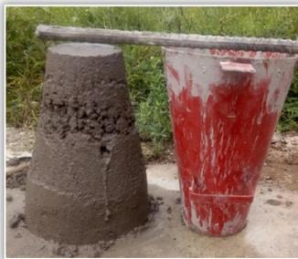
Figure 3. Concrete workability test using slump cone
