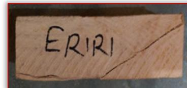
Figure 2: Failure mode of 200mm (Splitting)
