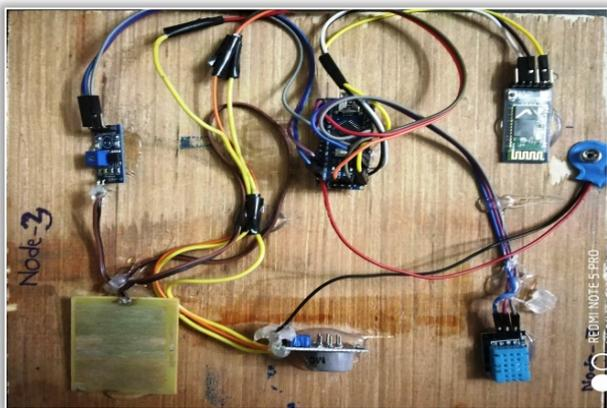
Figure 4. Node - 3 uses Bluetooth Communication
