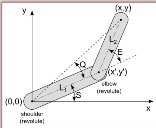
Figure 2: Trigonometry angles of SCARA inverse kinematics [9]
