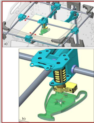
Figure 9. Machine simulation according to the given tool path within the last layer in PTC Creo environment
