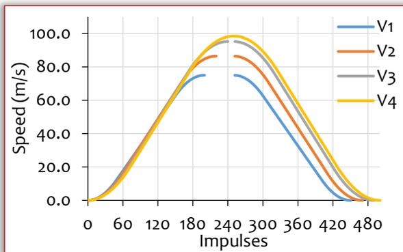
Figure 7: Comparison of different S velocity profiles
