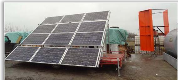
Figure 1. Mobile system for the production of electricity from alternative sources (solar + wind) for agricultural applications and monitoring, tele-transmission and crop management services
