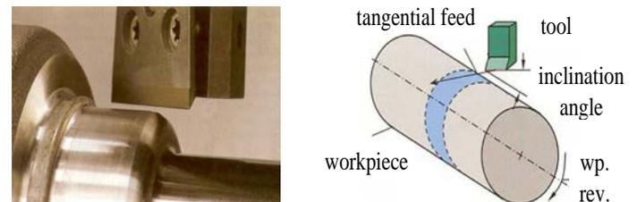
Figure 1. Tangential turning and its kinematic scheme [14]
