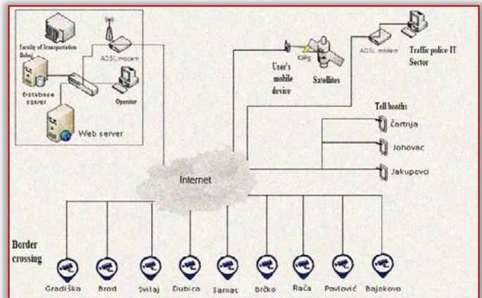
Figure 4. Architecture of distributed information communication system for traffic monitoring and actively informing traffic participants
