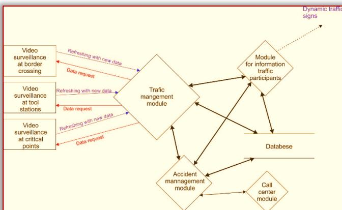
Figure 3. Structure and principle of operation of acquisition part of the system
