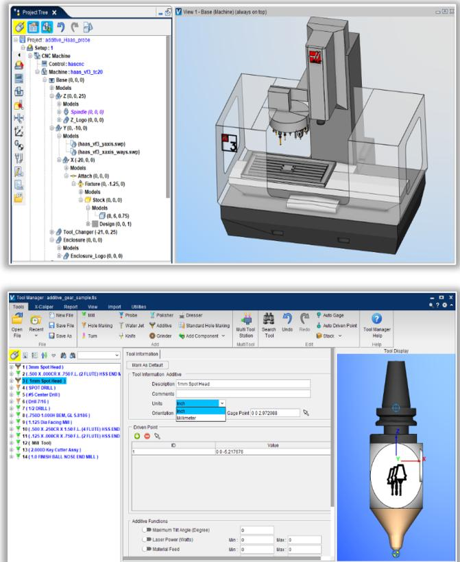
Figure 5. Selected virtual machine Haas vF3 and Laser DED extruder
