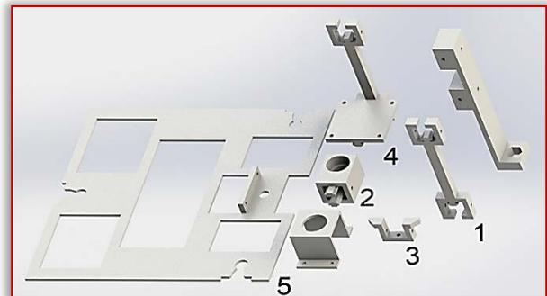
Figure 8: Solidworks CAD models of 3D printed components
