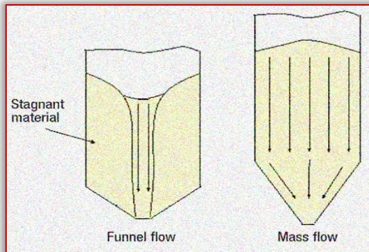
Figure 1 – Two types of flow patterns can occur when a bulk solid is discharged from a bunker, hopper, bin or silo: A typical funnel flow pattern is shown on the left, and a mass flow pattern is shown on the right (Jenike A.W., 1964)
