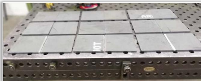
Figure 2. Plates prepared for welding
