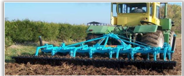
Figure 6. Chisel, PC 13
