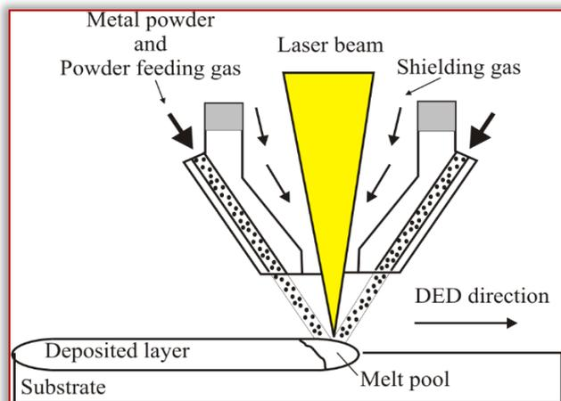
Figure 2. Schematic of a Laser powder DED process
