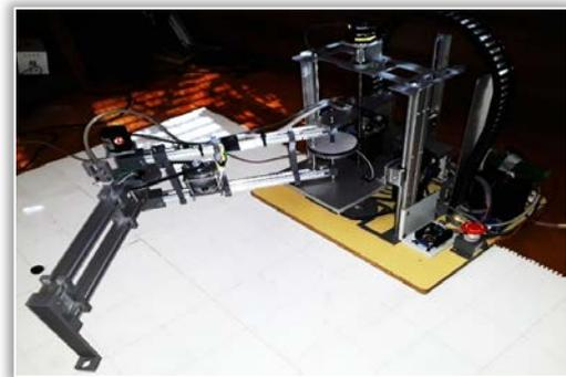
Figure 14: Final look of the SCARA robotic arm
