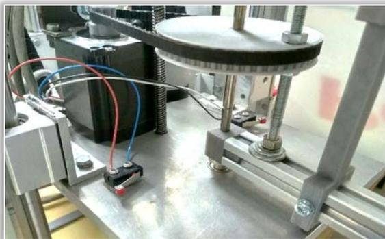
Figure 11: Pulley and motor assembly for shoulder
