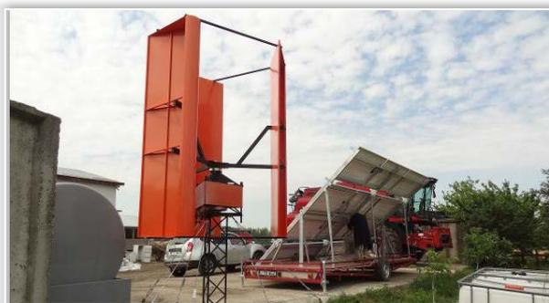
Figure 3. Vertical axis wind turbine
