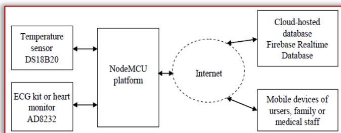
Figure 4. Block scheme of the solution
