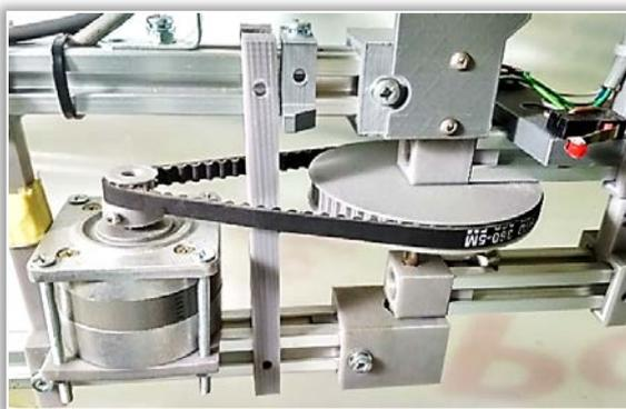
Figure 12: Pulley and motor assembly for elbow
