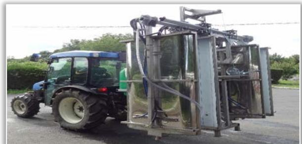
Figure 17. Spraying machine in vine plantations
