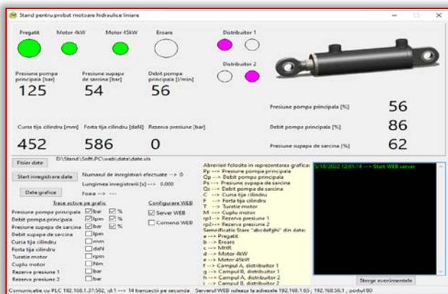
Figure 4. The main panel of the PC application
