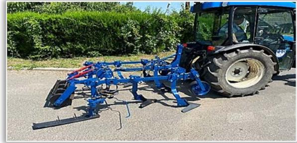
Figure 16. Weeding equipment for working in rows and between the vine trunks, EPV 2.2
