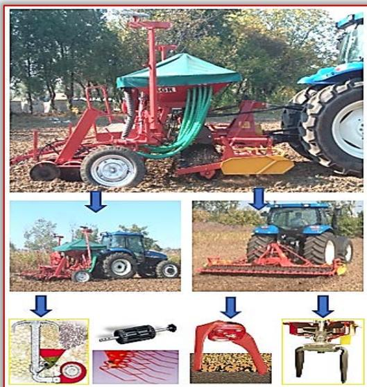
Figure 10. Technical equipment with working bodies for preparing the soil and sowing grassy cereals
