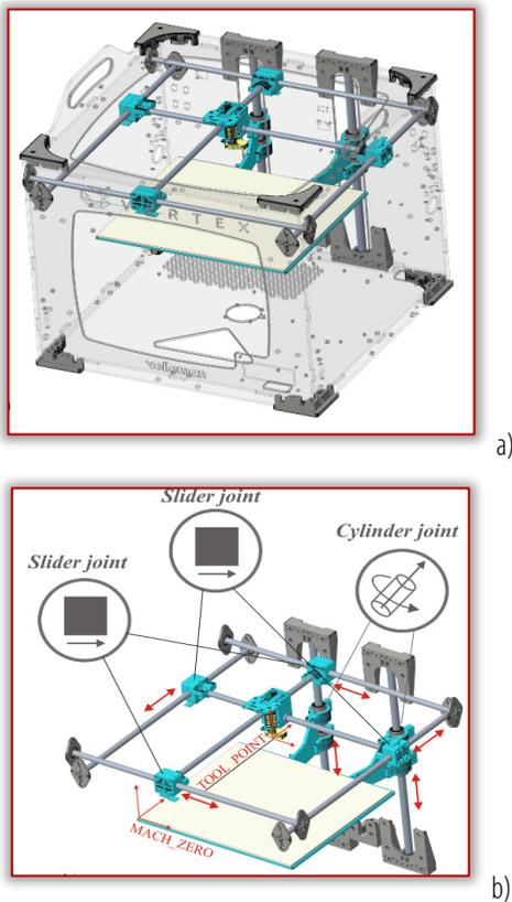
Figure 4. Virtual machine Velleman Vertex K8400 with defined kinematic connections and coordinate systems
