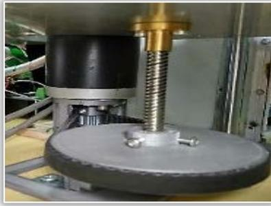
Figure 10: DC motor connected to a threaded rod via belt and pulley mechanism
