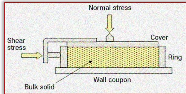
Figure 2 – By measuring the force required to slide a sample of powder along a wall coupon, the angle of wall friction can be determined (Mehos G., 2016)
