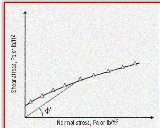
Figure 3 – The angle of wall friction ( $\phi'$ ) is determined by drawing a line between the wall yield locus (which is constructed by plotting shear stress against normal stress), and the origin, as shown here  $\Delta, \phi'$ . (Mehos G., 2016)
