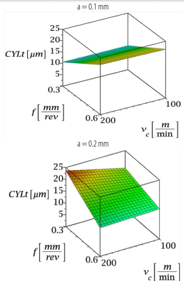
Figure 2. Cylindricity error (CYLt) as a function of the technological parameters
