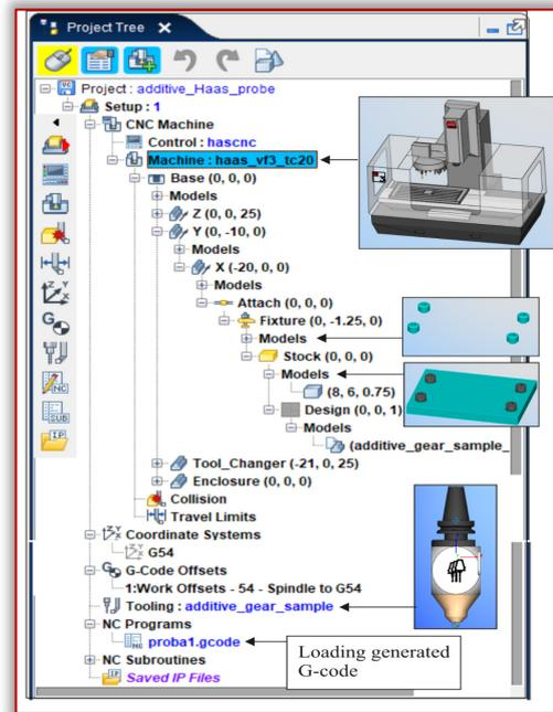
Figure11. VERICUT project hierarchical tree, an example of for additive technology
