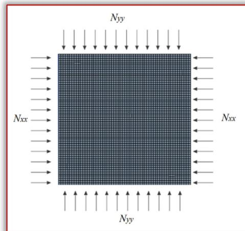
Figure 3. Composite plate loaded by biaxial compression load
