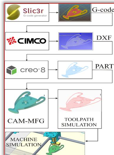
Figure 8. Procedure for indirect machine simulation of additive tool path on each layer An illustration of the work done on Velleman Vertex K8400 during 3D printing of the first example is shown in Figure10.
