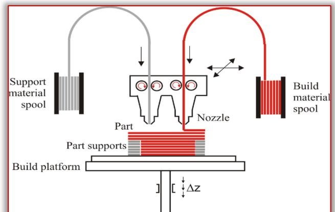
Figure 1. Schematic of FDM system
