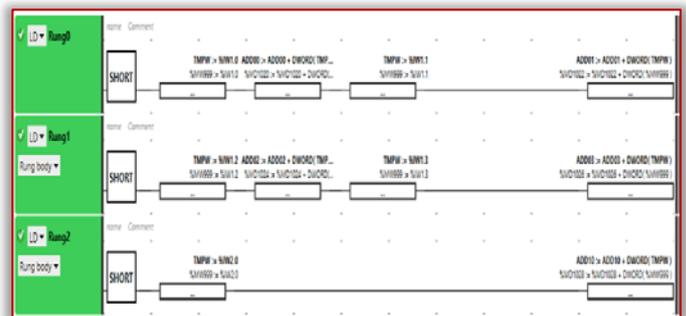
Figure 5. Ladder diagram for data acquisition from stand transmitters
