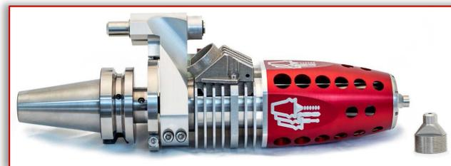
Figure 3. Laser DED extruder in a testing setup
