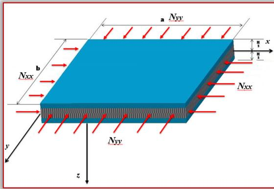
Figure 1. Symmetric square composite plate with 4 plies
