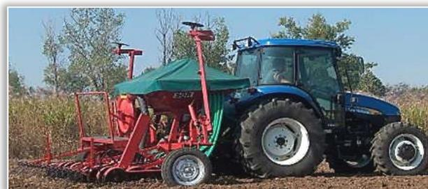
Figure 13. Mechanical–pneumatic seeder
