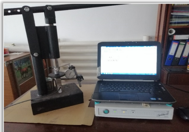
Figure 3 – Test equipment for determining the compressive strength of granular fertilizer material based on biosolids
