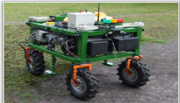
Figure 8 – Autonomous weed control robot "Weedy" designed at the University of Osnabrück, Germany (Macrii et al. 2022)
