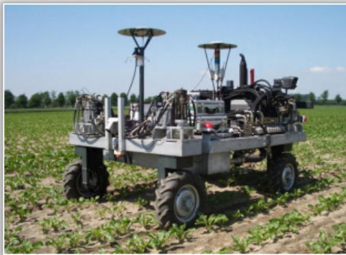
Figure 6 – Autonomous weed-fighting robot designed at Wageningen University, Netherlands (Boris et al. 2022)
