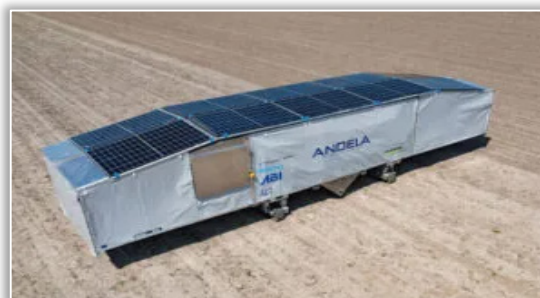
Figure 12 – The autonomous weeding robot is 9 meters wide and has 12 weeding units. On the roof are solar panels for electric motors.
