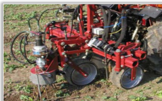
Figure 3 – “Querhacke” cycloidal harrow designed at the University of Osnabrück, Germany (Gruľová et al. 2020)
